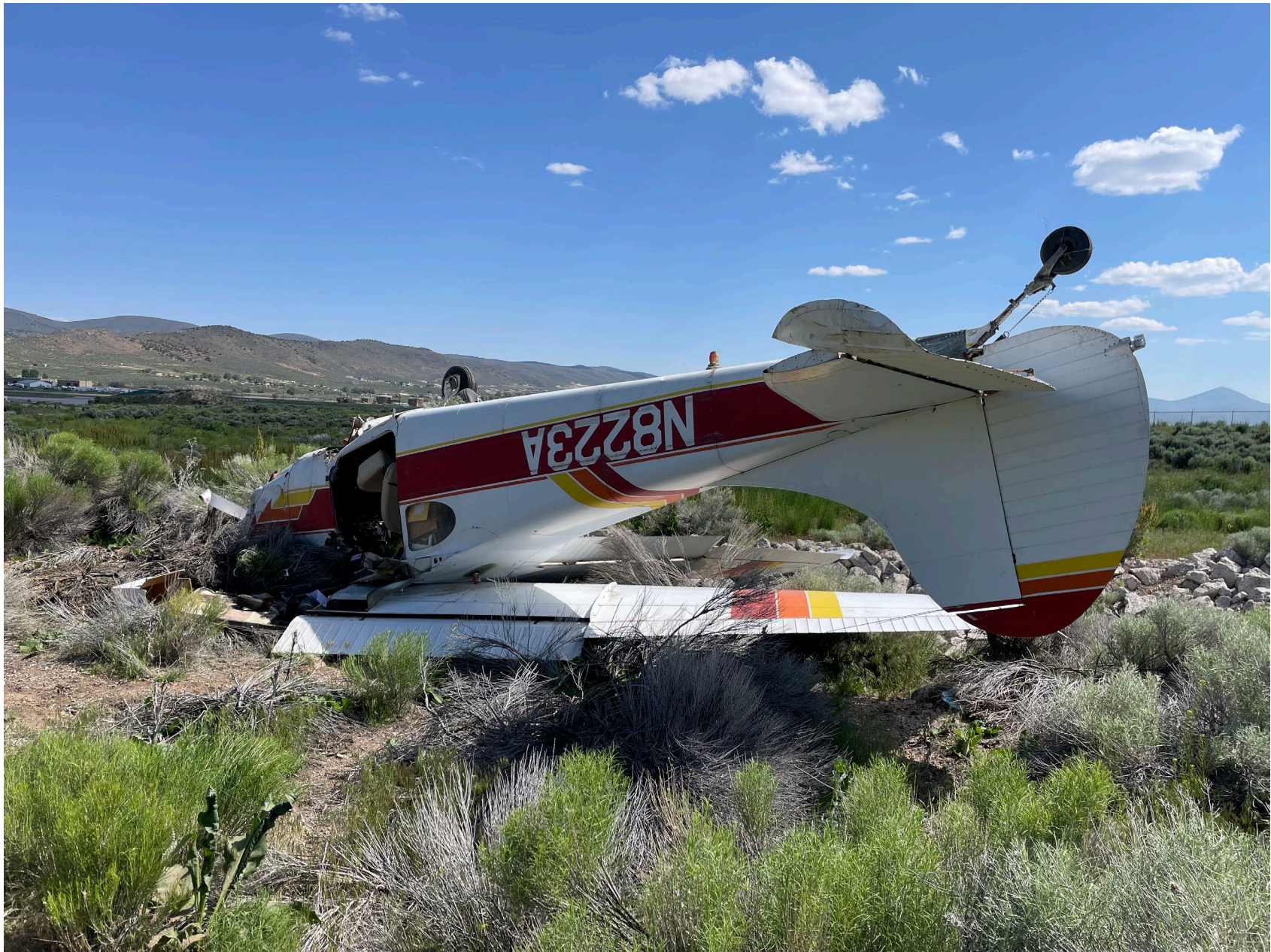
Photo 2 - View of Damage to Fuselage, Wings, and Elevator (Source: Airport Security Coordinator)
