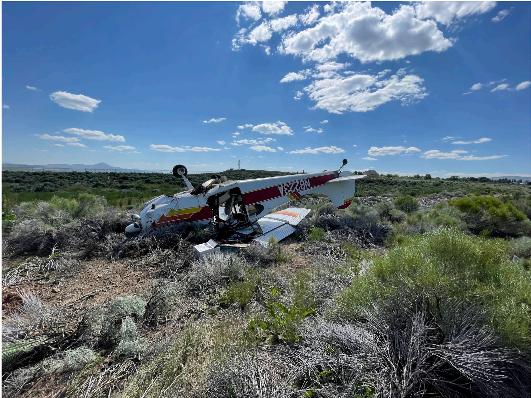
Photo 1 – View of Damage to Fuselage, Wings, and Elevator (Source: Airport Security Coordinator)
