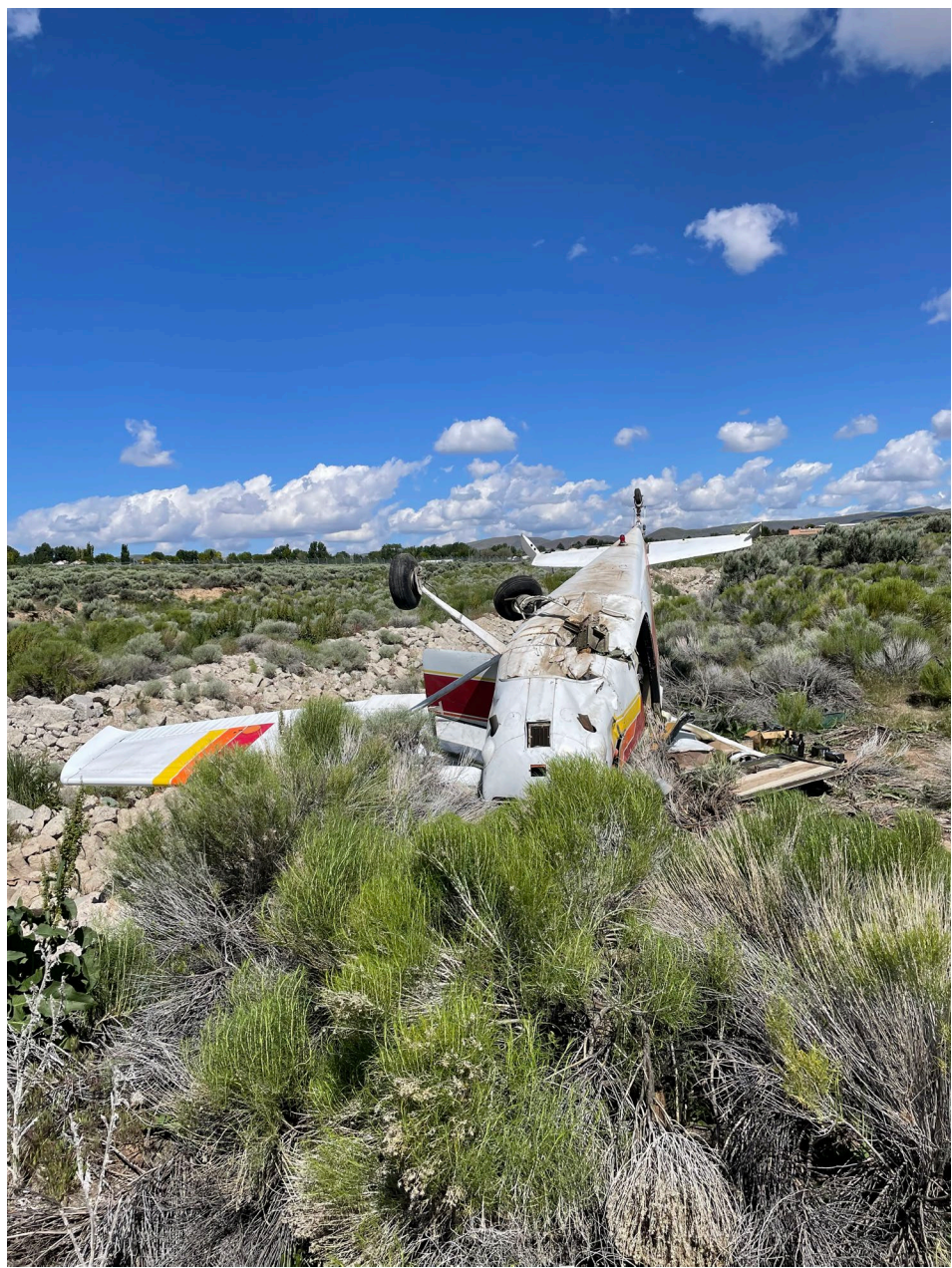
Photo 3 – View of Damage to Fuselage, Wings, and Elevator (Source: Airport Security Coordinator)
