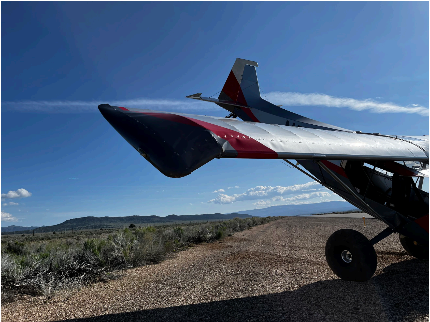
Photo 1 – View of right wing damage. (Photo courtesy of pilot)
