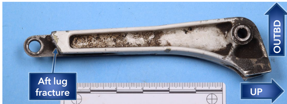
Figure 1. Overall view of the forward side of the submitted side brace lock bellcrank as received.
