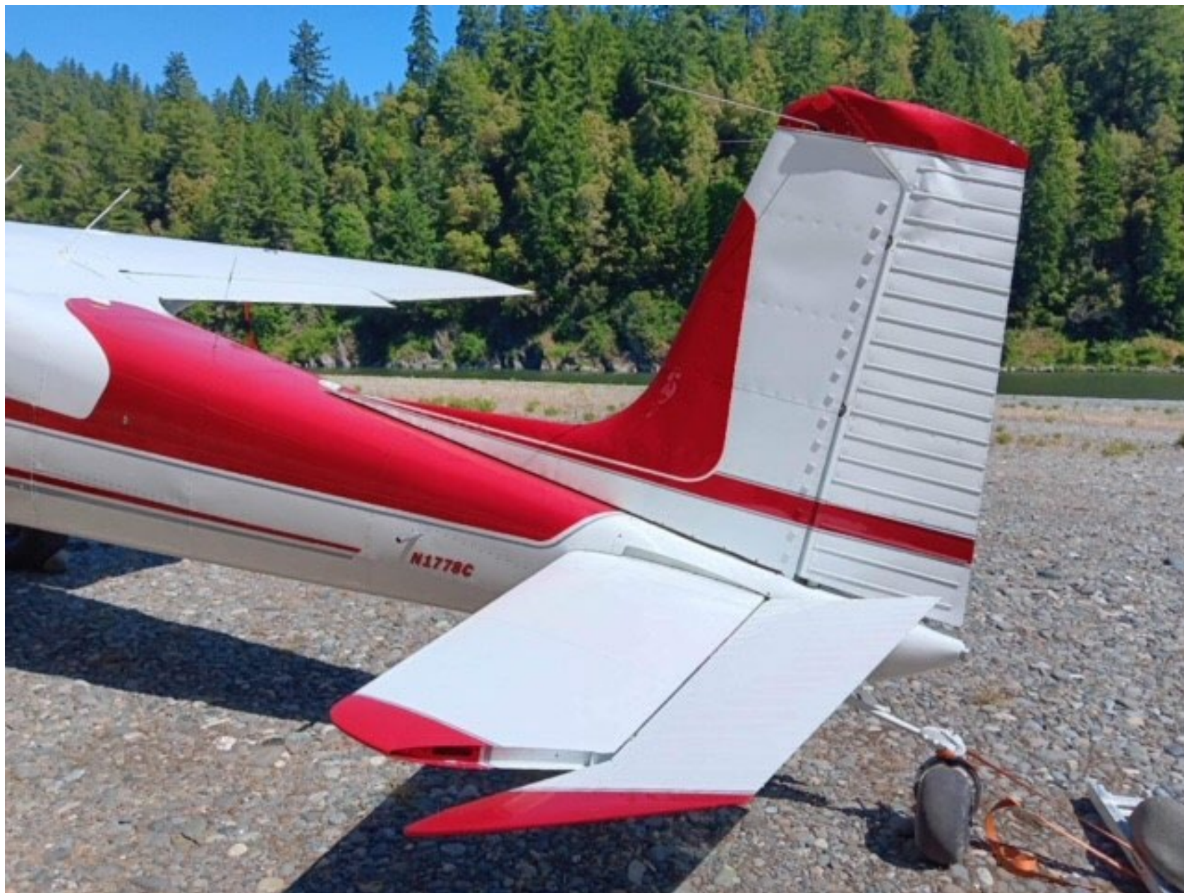
Photo 1 – View of damage to rudder (courtesy of pilot)
