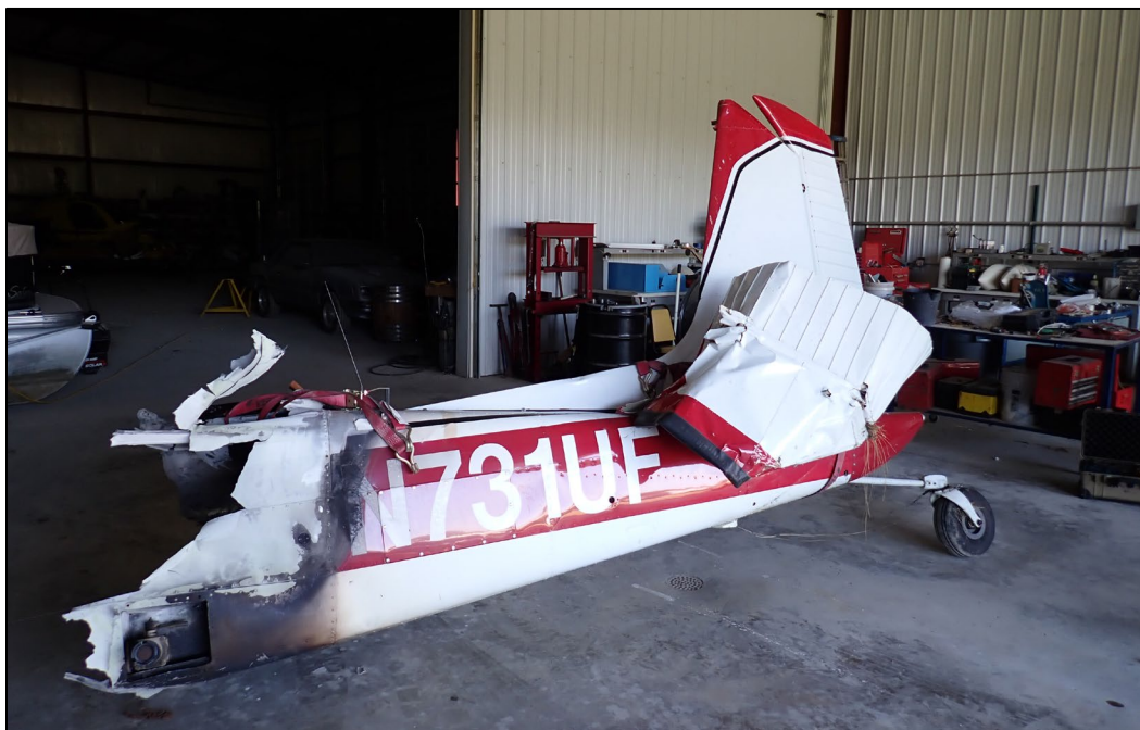
Figure 2: View of empennage damage (photo courtesy of Textron Aviation)
