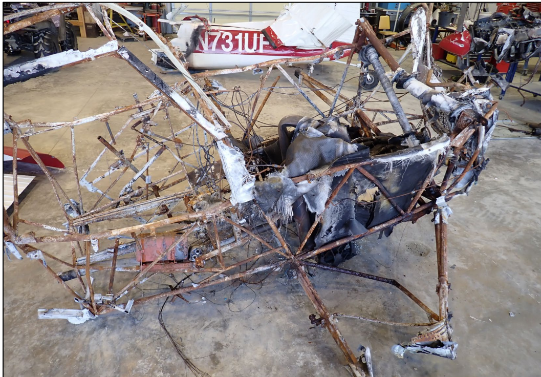
Figure 1: View of fire damage to cockpit (photo courtesy of Textron Aviation)
