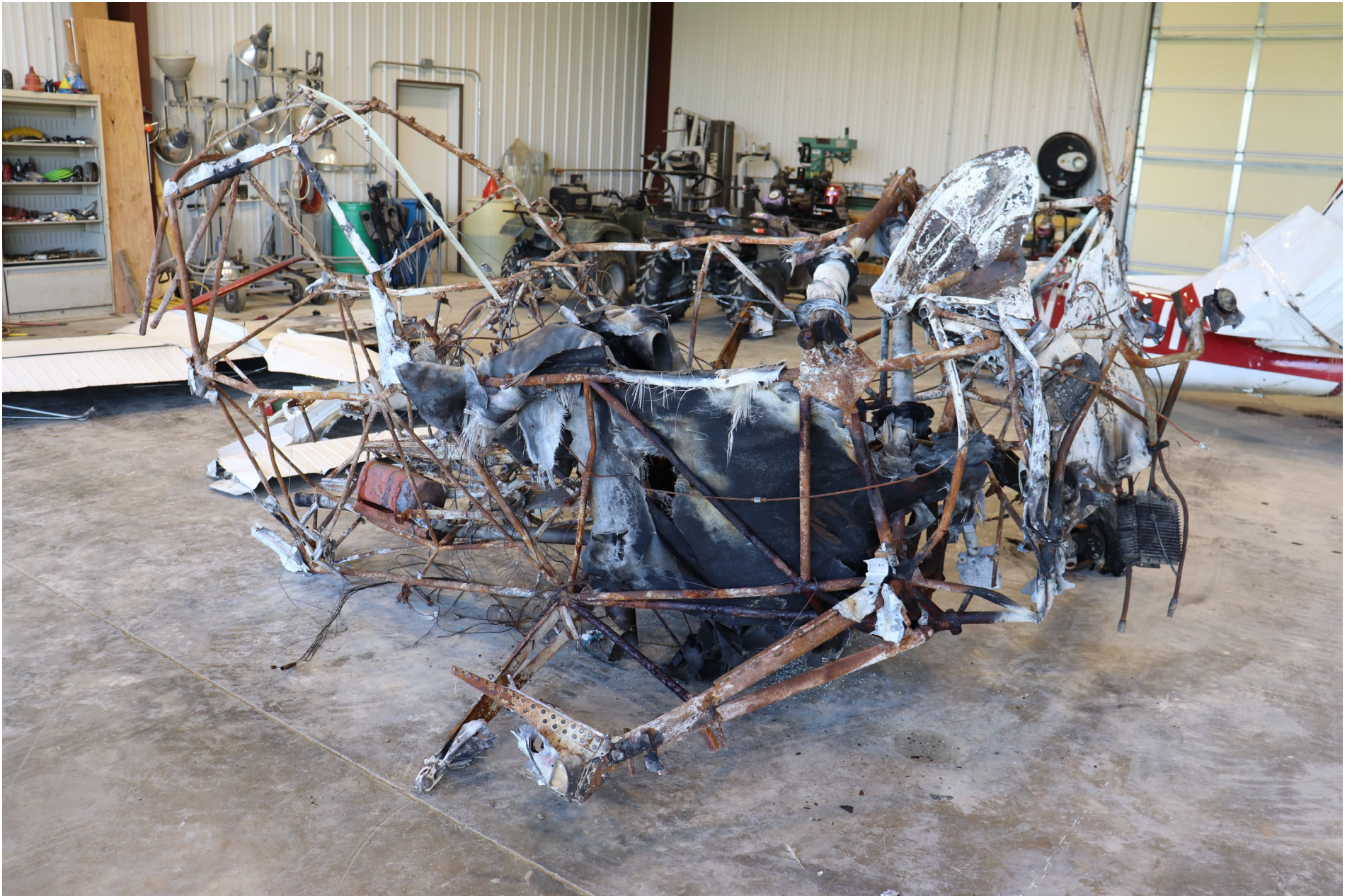
Photo 3 – View of cockpit fire damage
