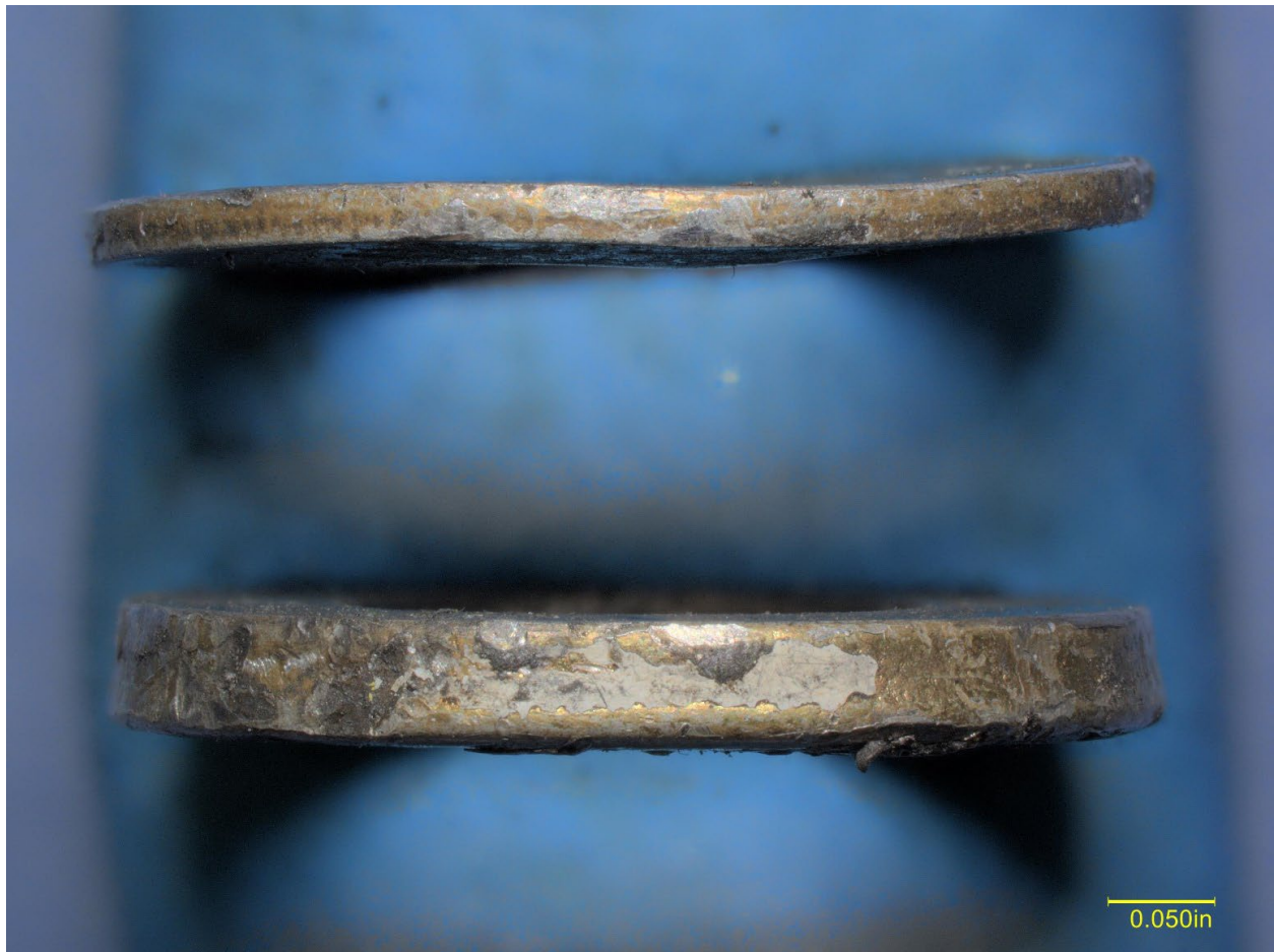
Figure 8. Digital microscope image showing the profile of the washers that had been assembled to the upper torque link bolt.
