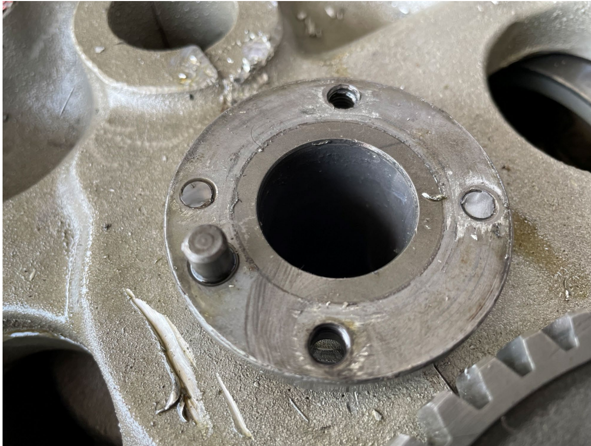
Photograph 5 - Crankshaft Gear Bolt Damage (Courtesy of NTSB)
