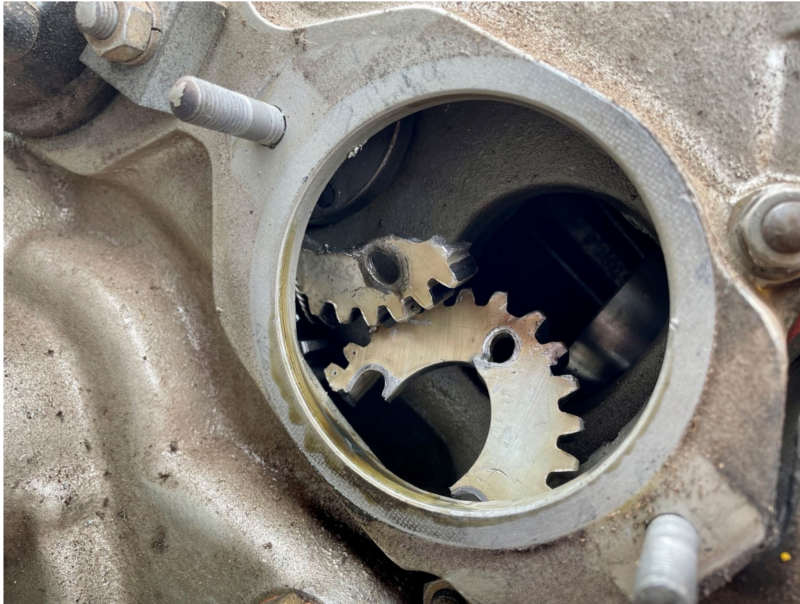
Photograph 4 - Broken Crankshaft Gear in Accessory Case (Courtesy of NTSB)
