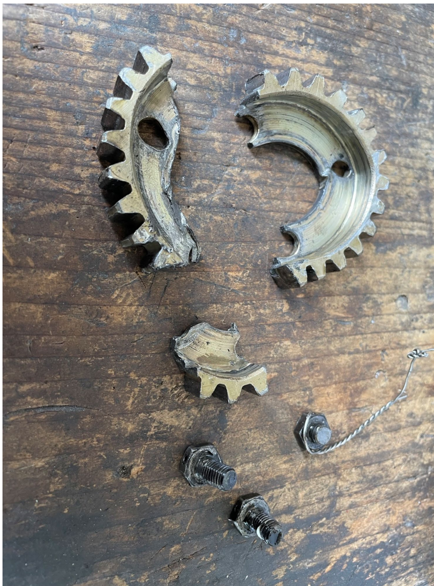
Photograph 6 - Camshaft Gear Fragments (Courtesy of NTSB)
