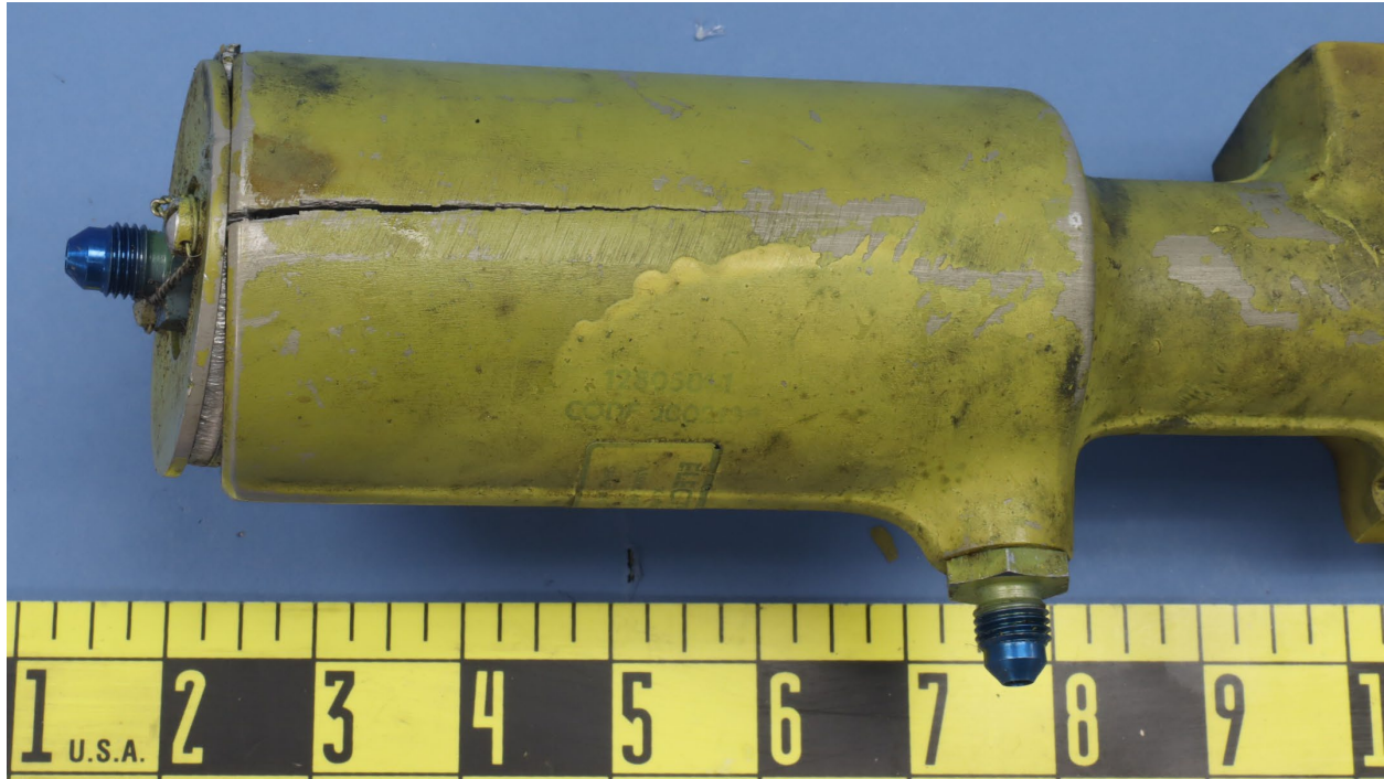
Figure 6. The longitudinal crack along the actuator housing barrel.
