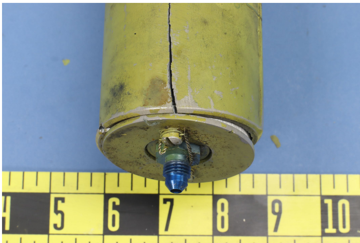
Figure 5. The longitudinal crack on the actuator housing, emanating from the circumferential crack (opposite the view in Figure 4a).
