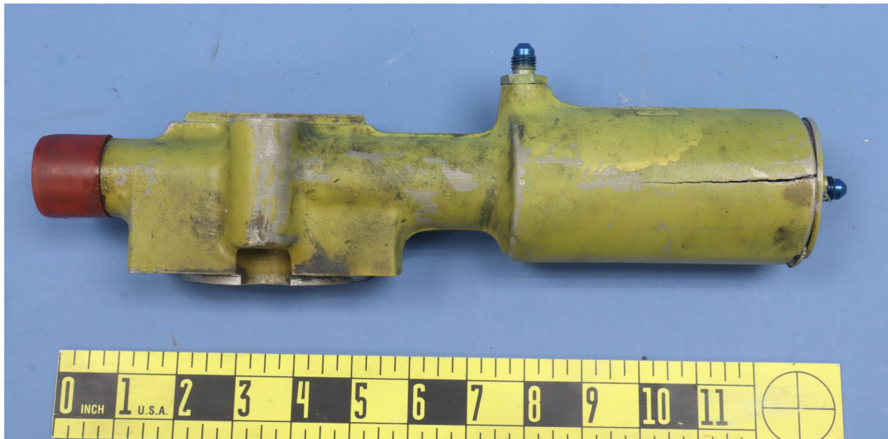
Figure 2. View of the hydraulic actuator, viewed opposite that in Figure 1b. This shows the longitudinal crack on the housing barrel.
