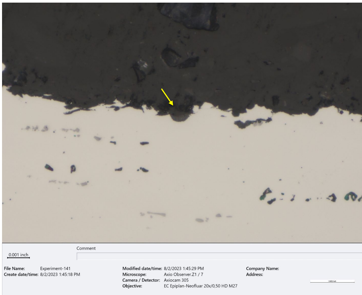
Figure 26. View of a corrosion pit (arrow) along the bottom surface of the groove shown in Figure 22 (~320X, as-polished).
