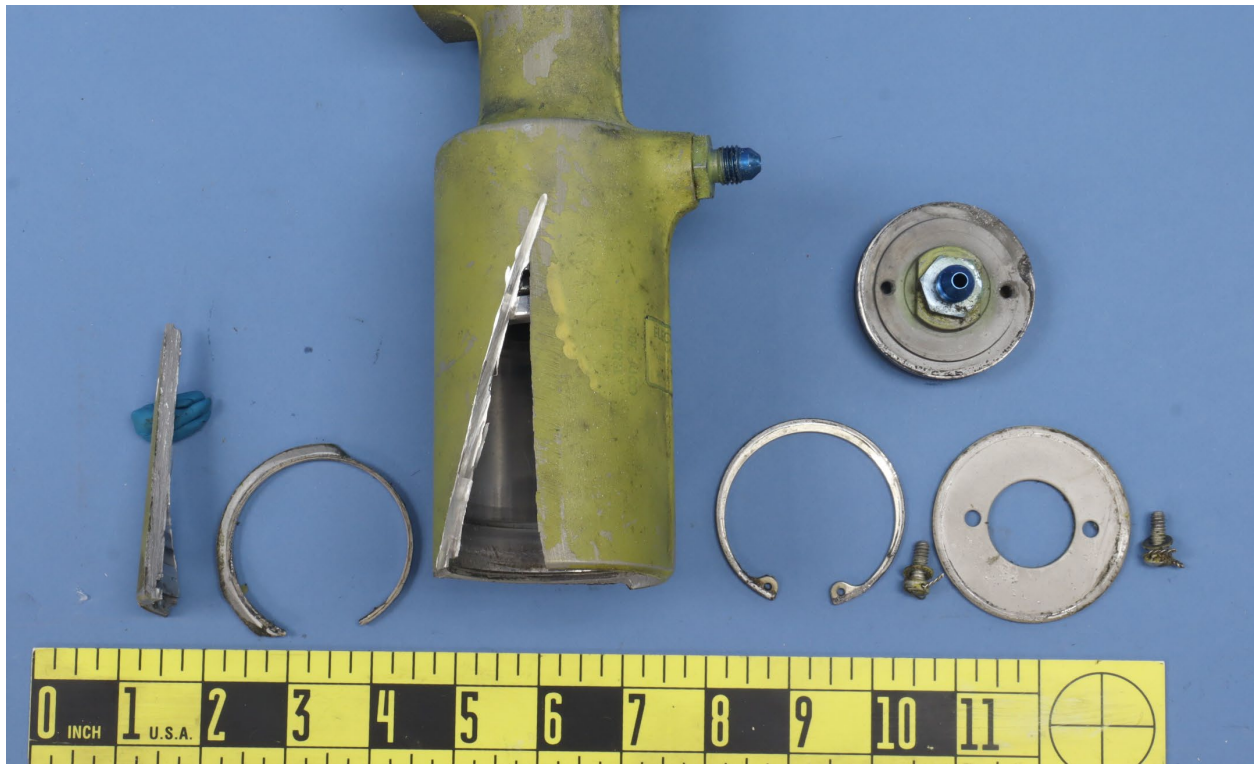
Figure 8. The cracked end of the actuator pictured in Figure 7a, after sectioning and removal of the cracked regions of the housing barrel.
