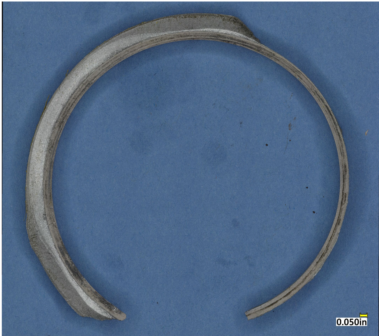
Figure 11. Montage of magnified images of the crack face of the circumferential crack, showing indications of progressive cracking.
