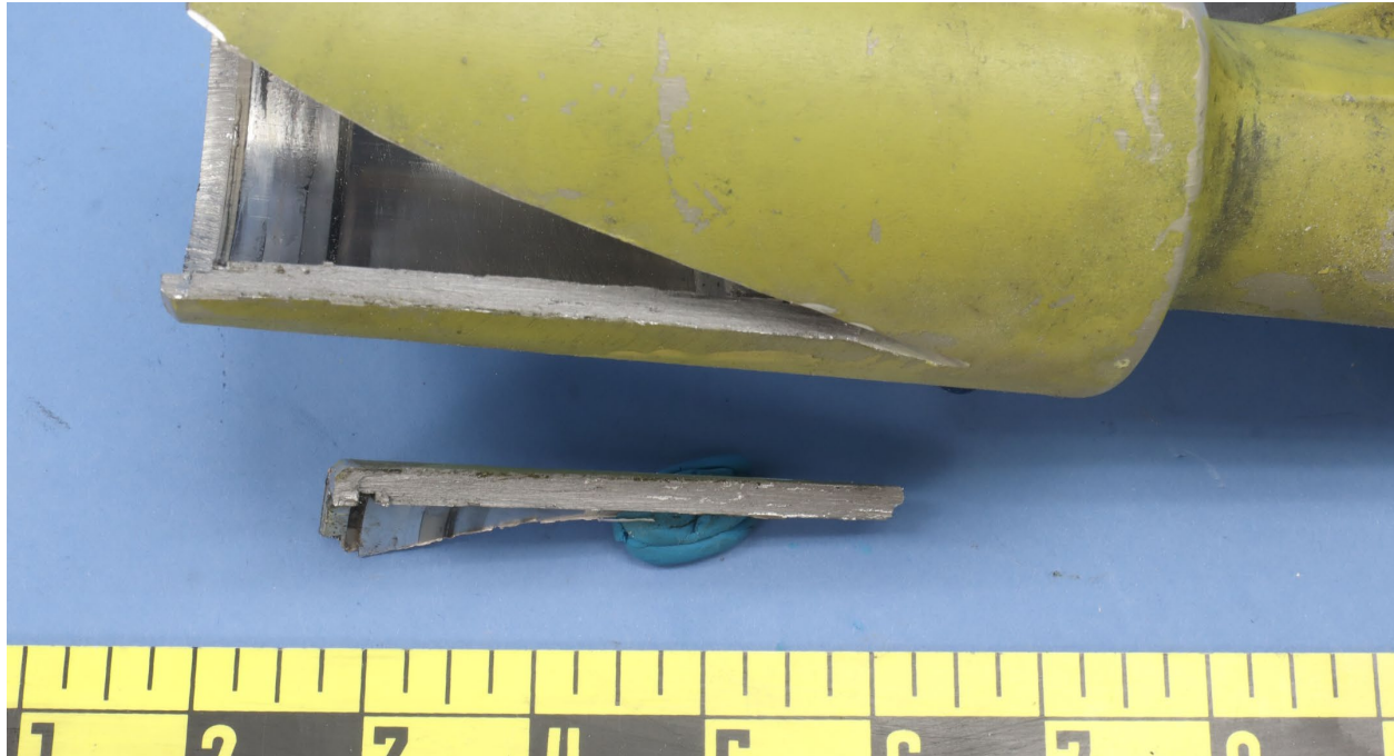
Figure 10. Mating faces of the longitudinal crack, after sectioning to open the crack faces.
