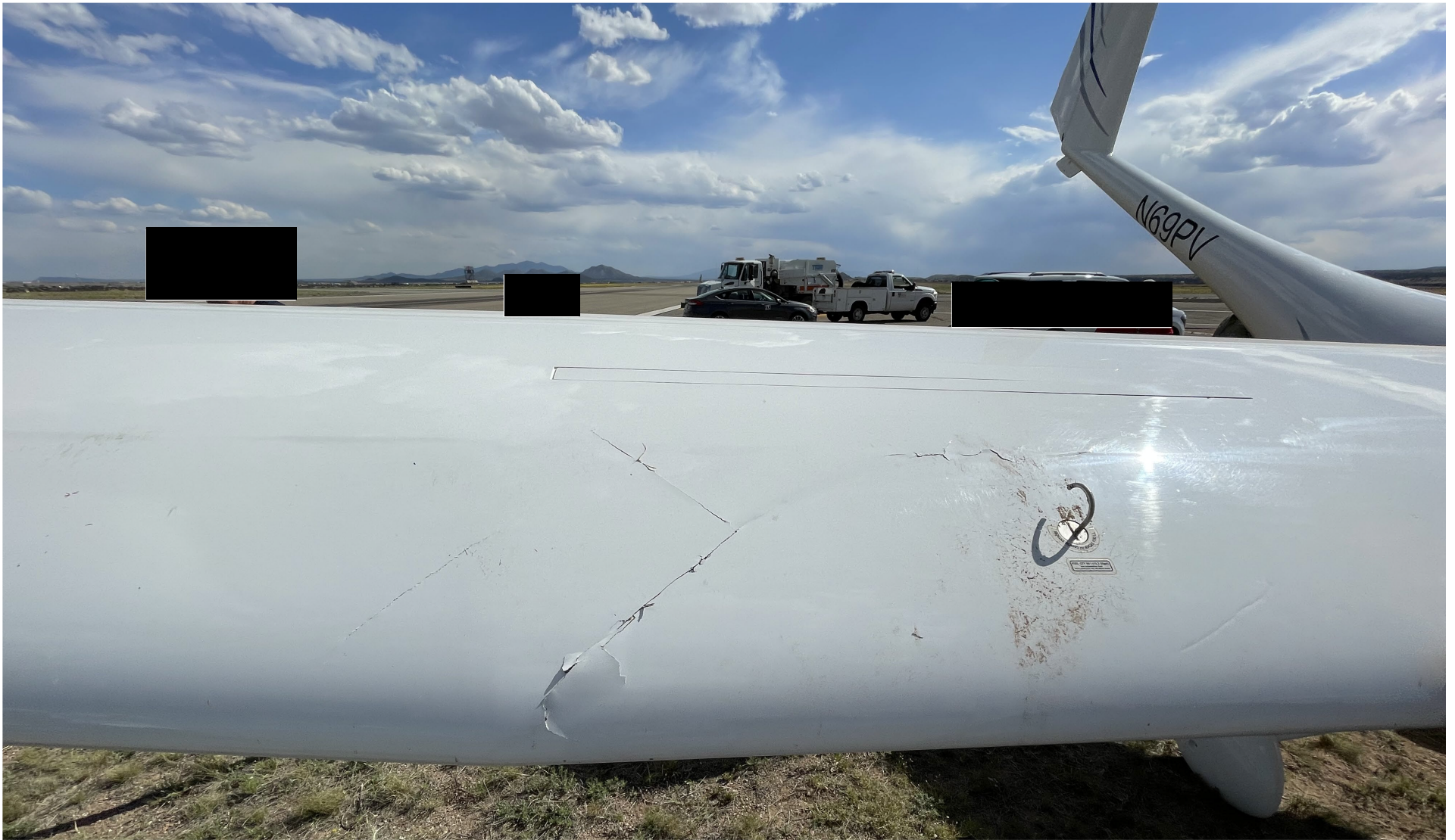
Photo 2 – View of damage to right wing (Courtesy of Owner)
