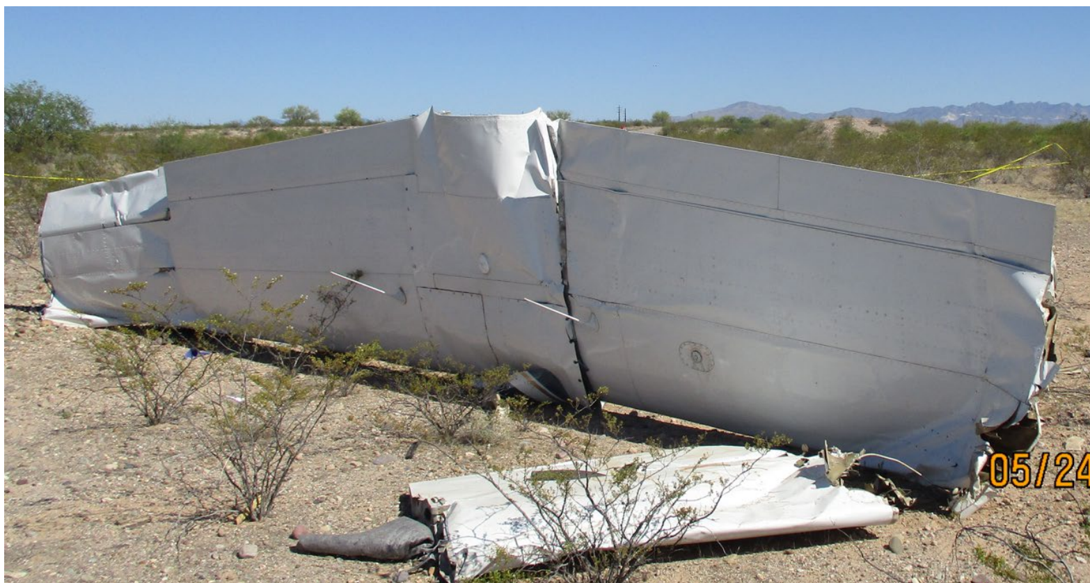
Photograph 2 - View of the damage to both wings (Courtesy of FAA)
