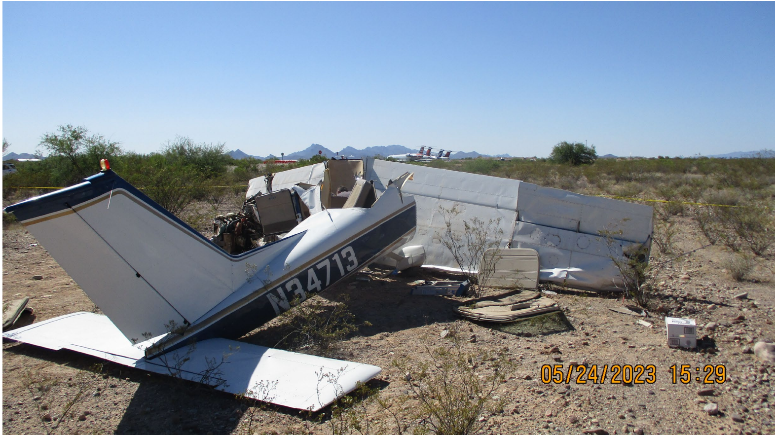
Photograph 4 - View of damage to the right side of the airplane (Courtesy of FAA)
