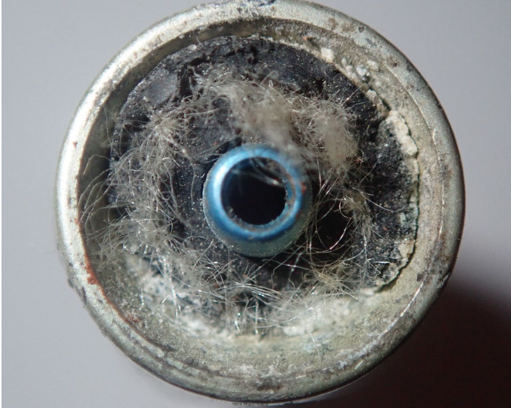
Figure 6 - Fuel pressure line with corrosion and brittle rubber
