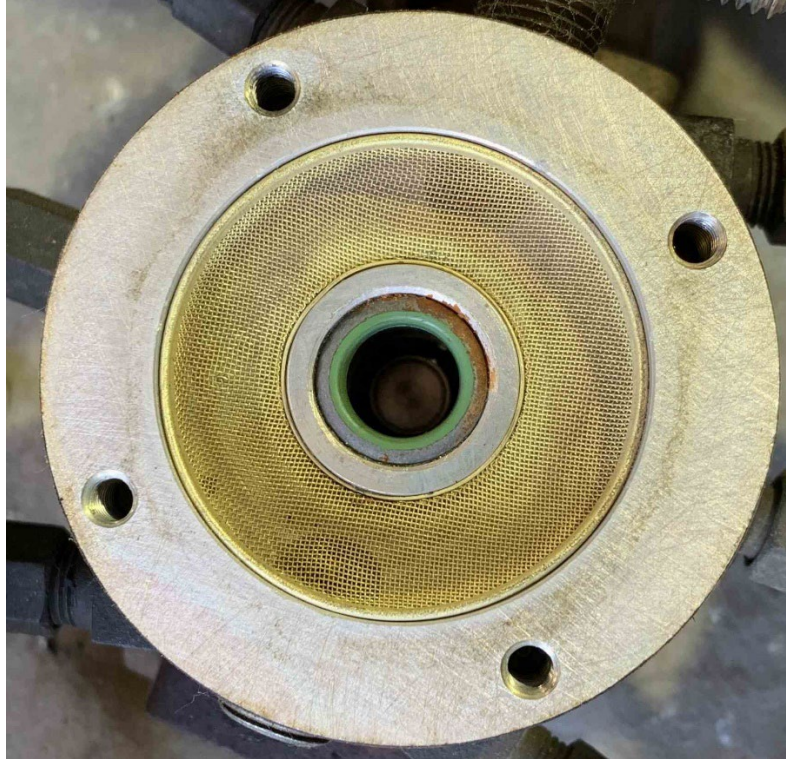
Figure 2 - Fuel manifold screen with corrosion
