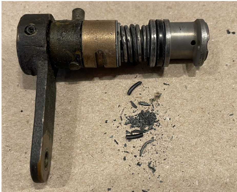
Figure 1 - Mixture control shaft with carbon deposits
