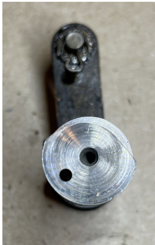
Figure 3 - Metering shaft mating surface with metering plug
