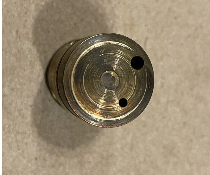
Figure 6 - Metering plug mating surface
