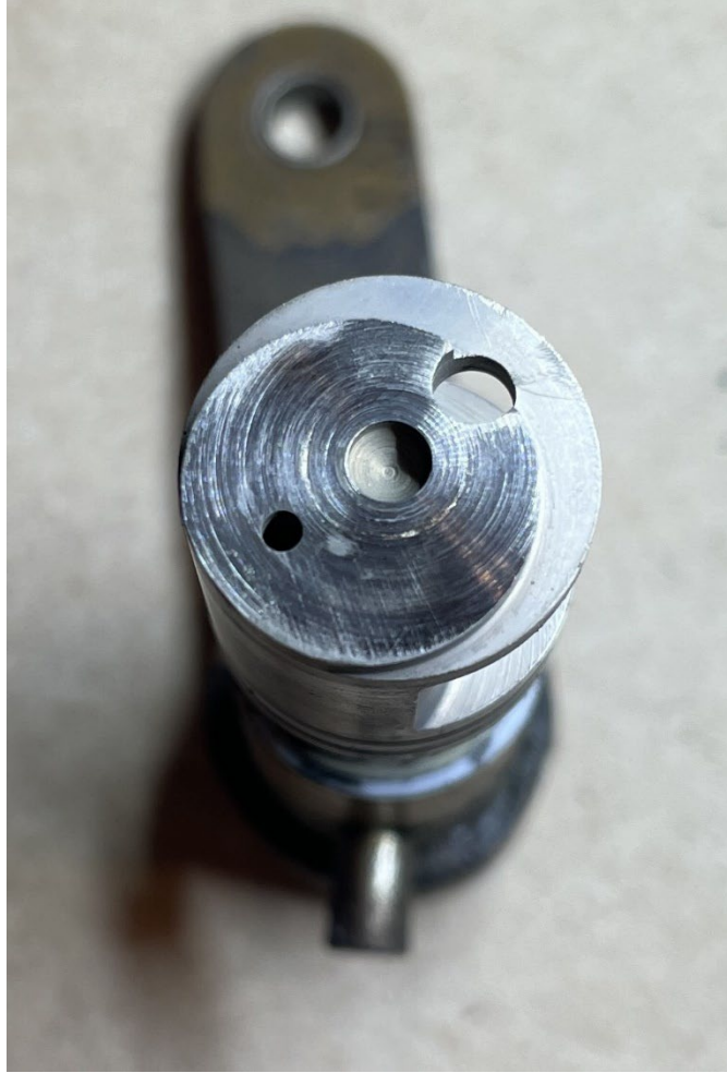
Figure 4 - Mixture shaft mating surface with metering plug
