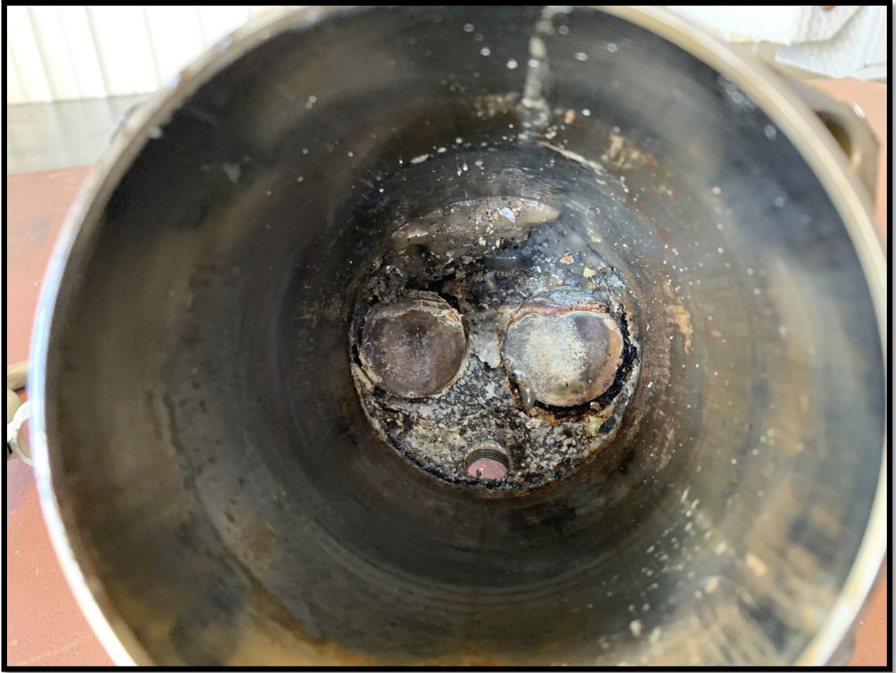
Figure 5. No. 4 stuck exhaust valve
