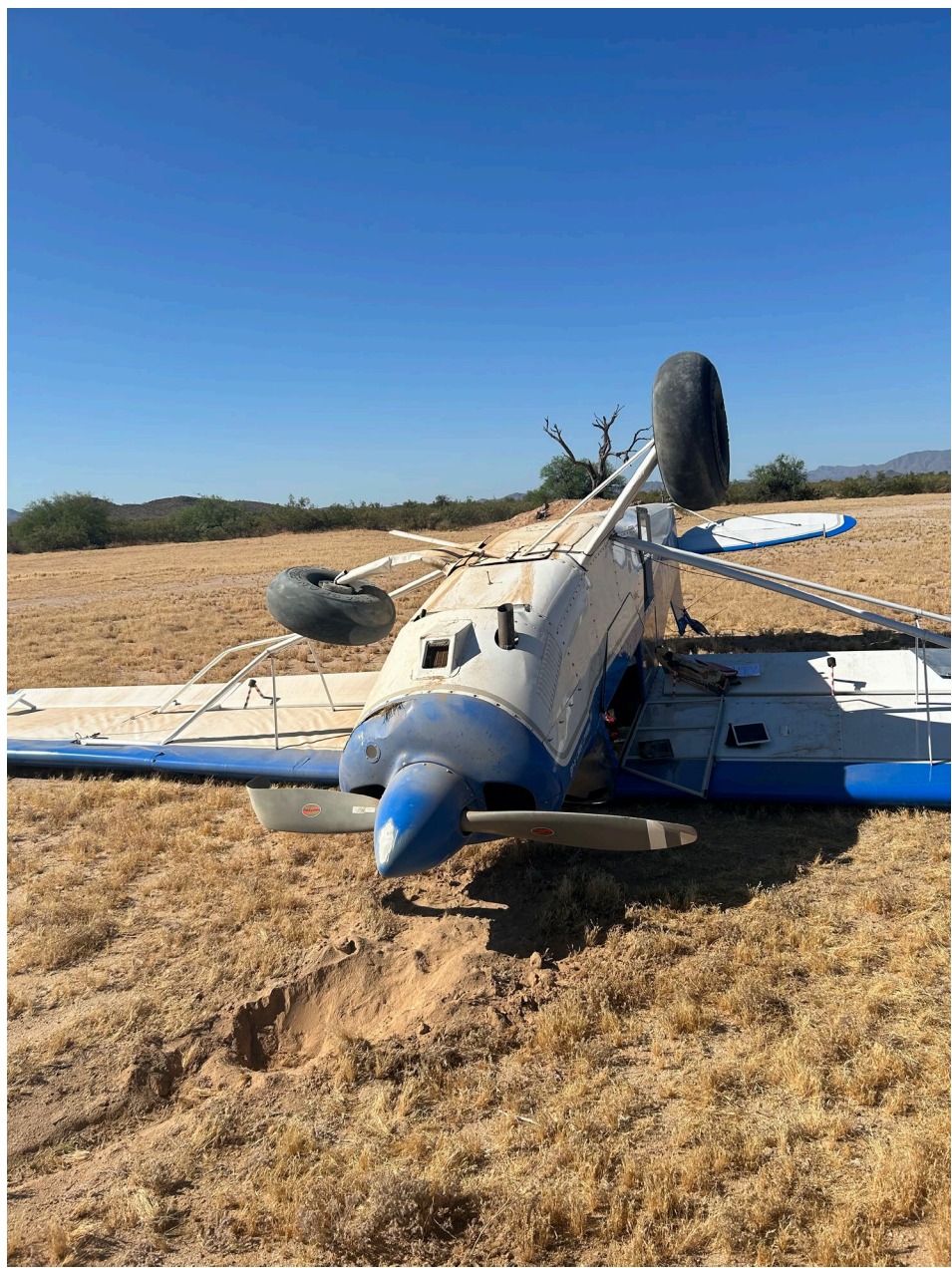
Photo 1 – View of damage to left wing struts (courtesy of pilot)
