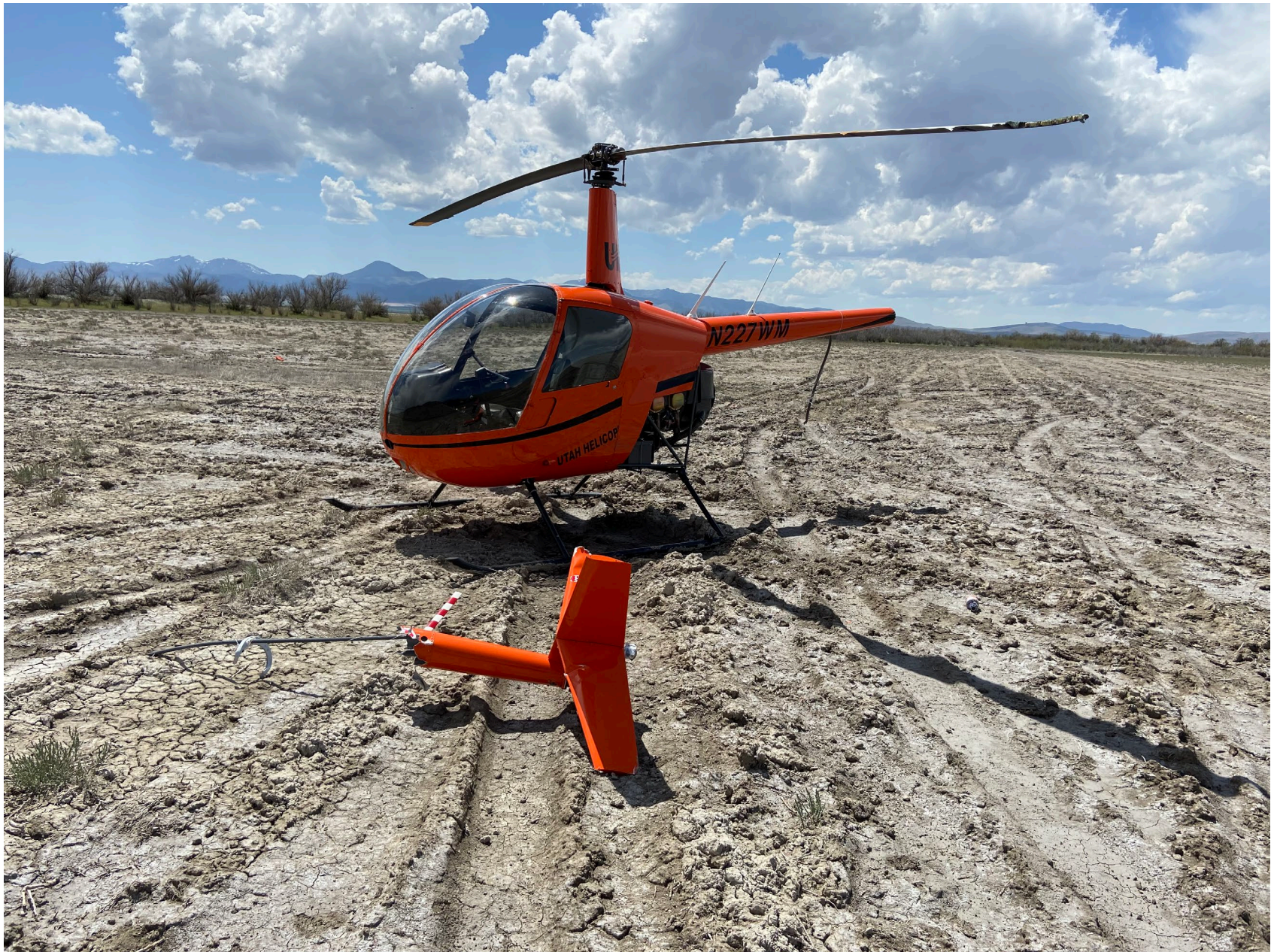
Photo 1 – View of helicopter with damage to main rotor blade, tailcone and tail rotor drive system (courtesy of the FAA)
