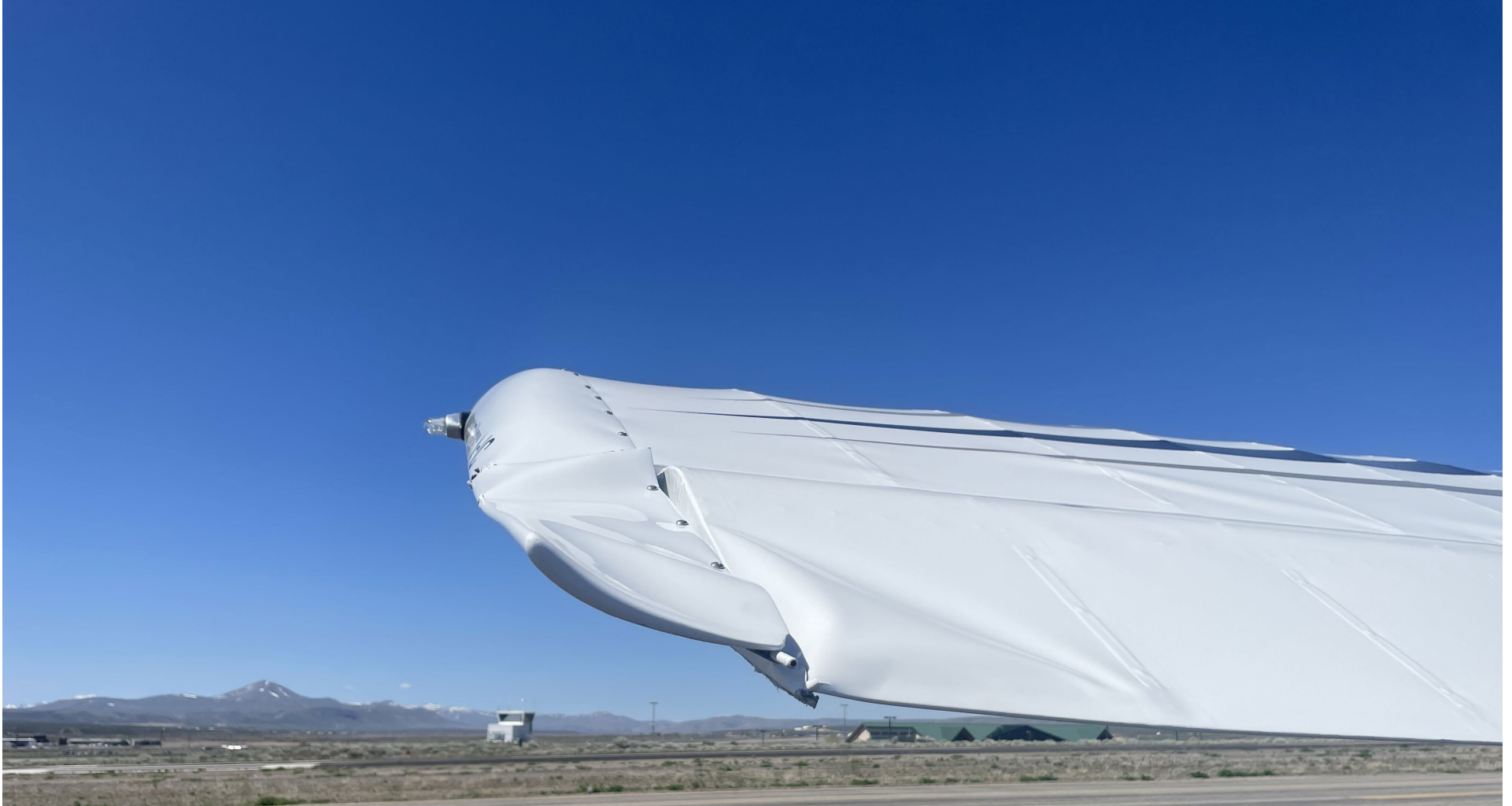
Photo 1 – View of damage to left aileron (Courtesy of Owner)
