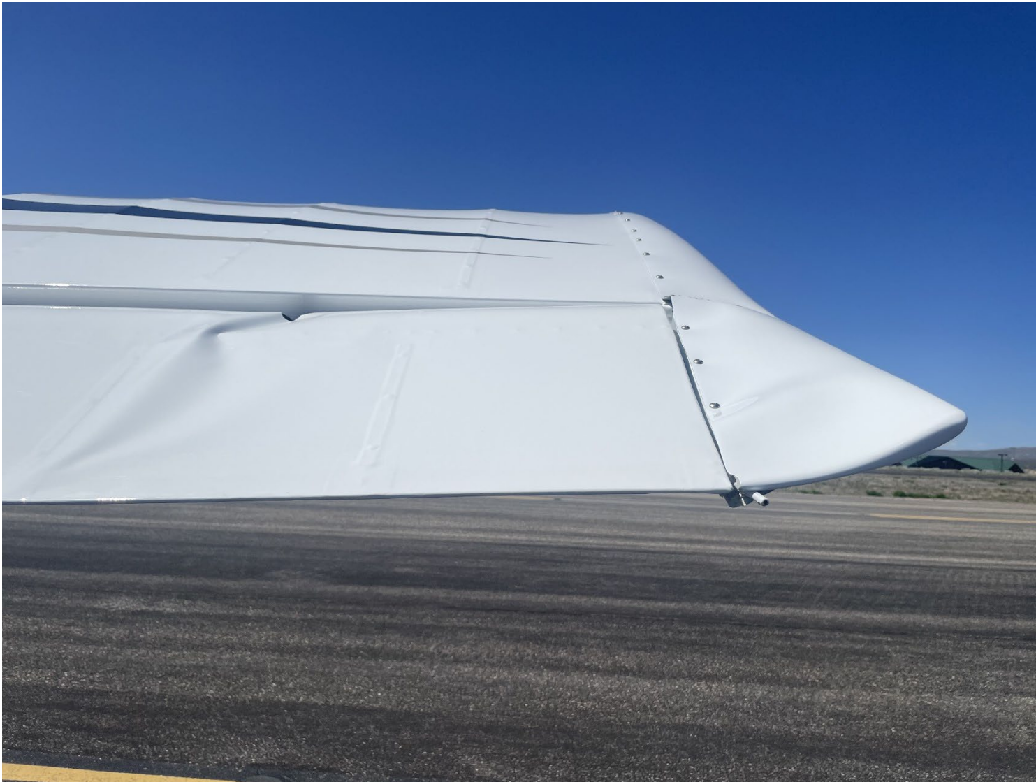
Photo 2 – View of damage to right aileron (Courtesy of Owner)
