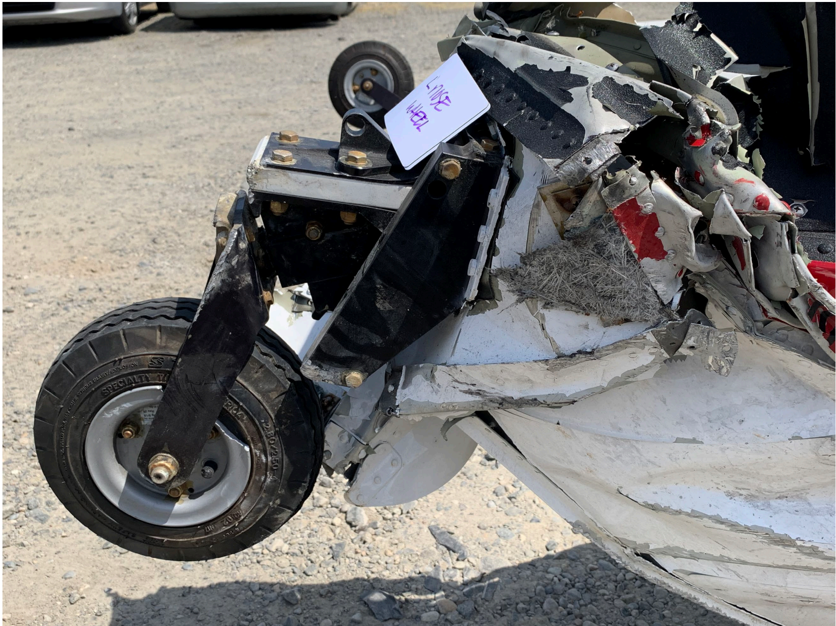
Photo 5 – View of Left Nose Wheel Retracted
