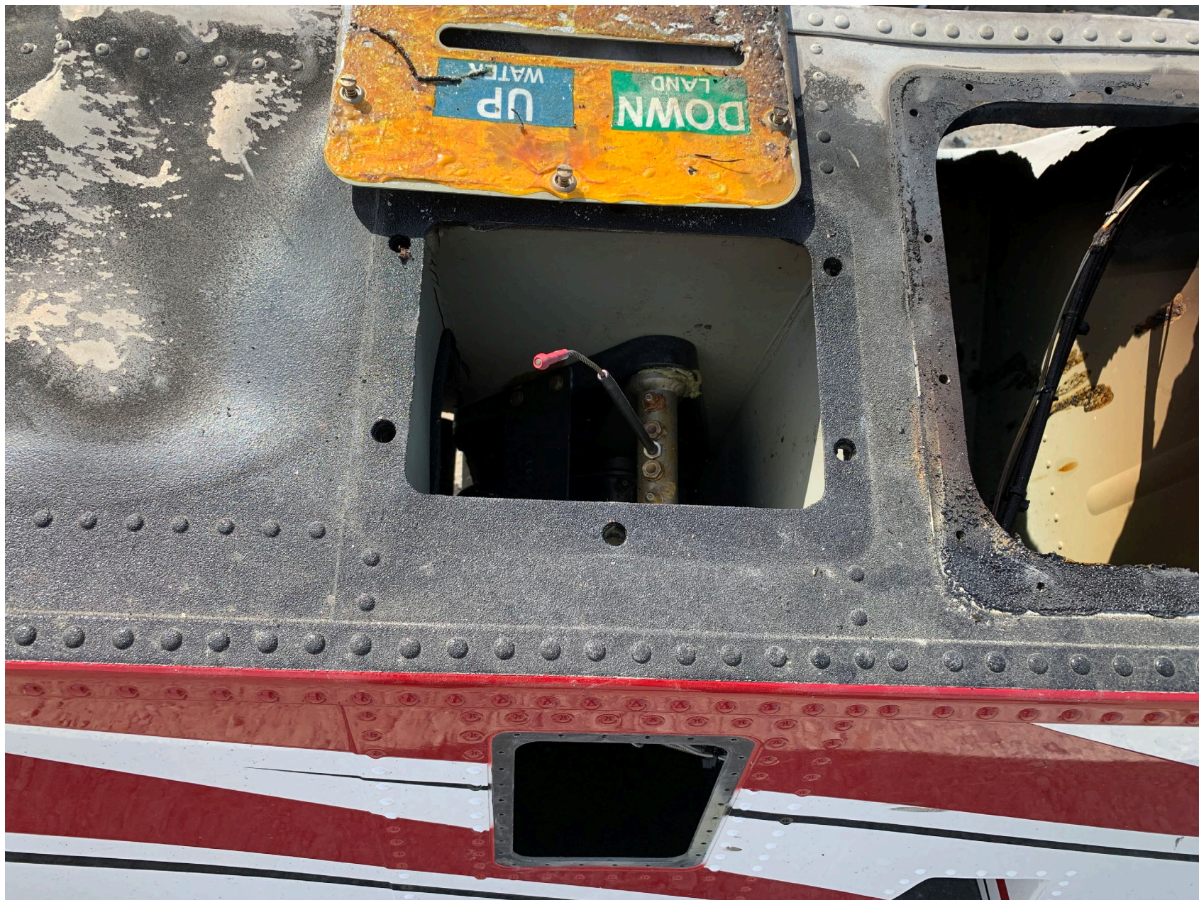
Photo 7 – View of Right Main Gear Actuator in the Retracted Position
