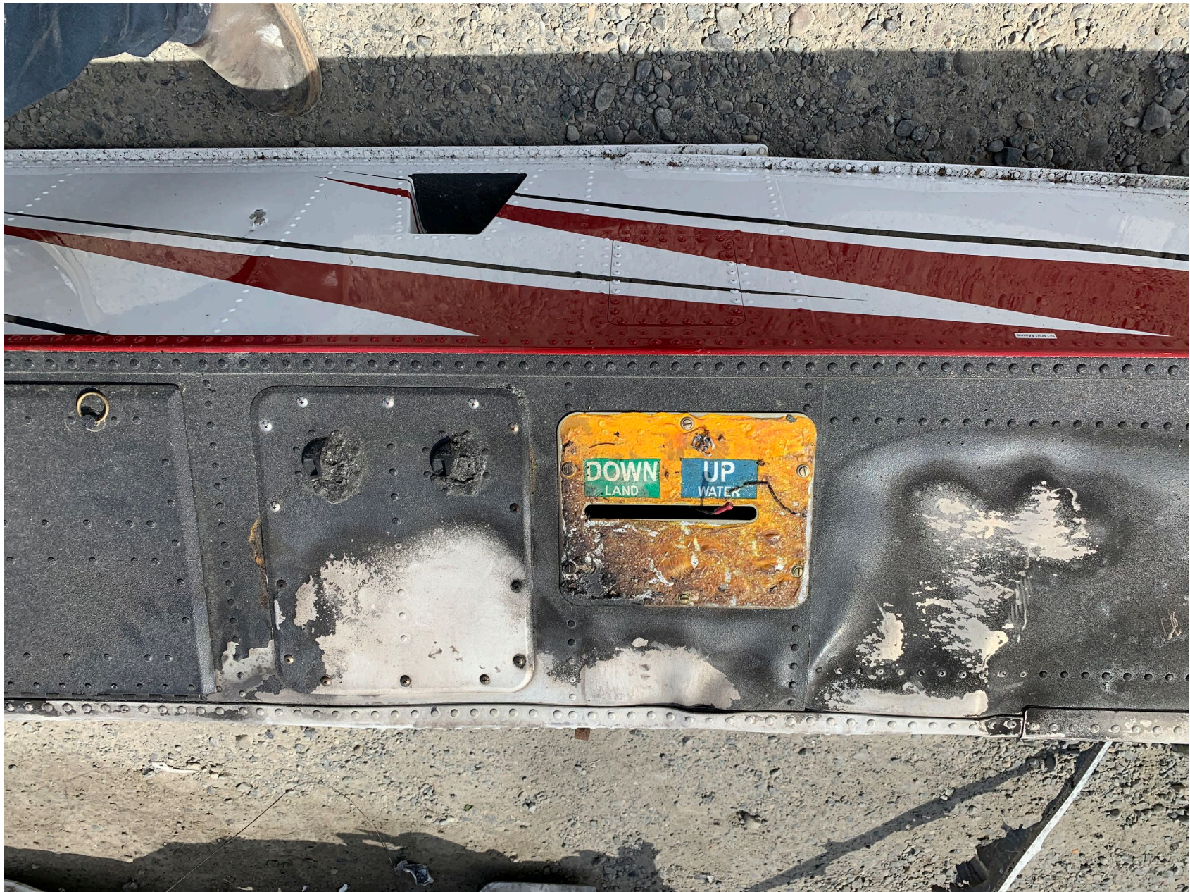
Photo 6 – View of Right Main Gear Indicator in the UP Position
