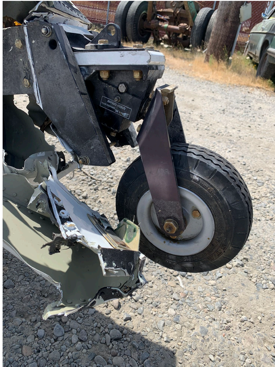
Photo 4 – View of Right Nose Wheel in the Retracted Position
