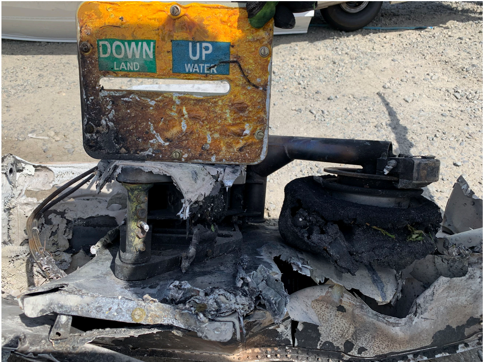
Photo 8 – View of Left Main Gear Actuator in the Retracted Position
