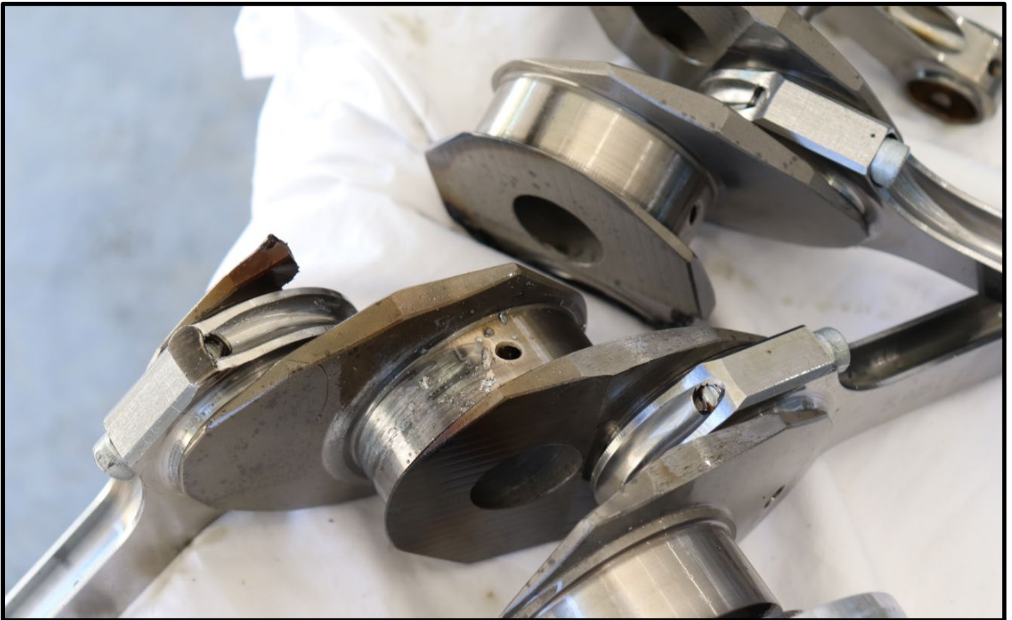
Figure 8: Journal Adjacent to Fracture Surface
