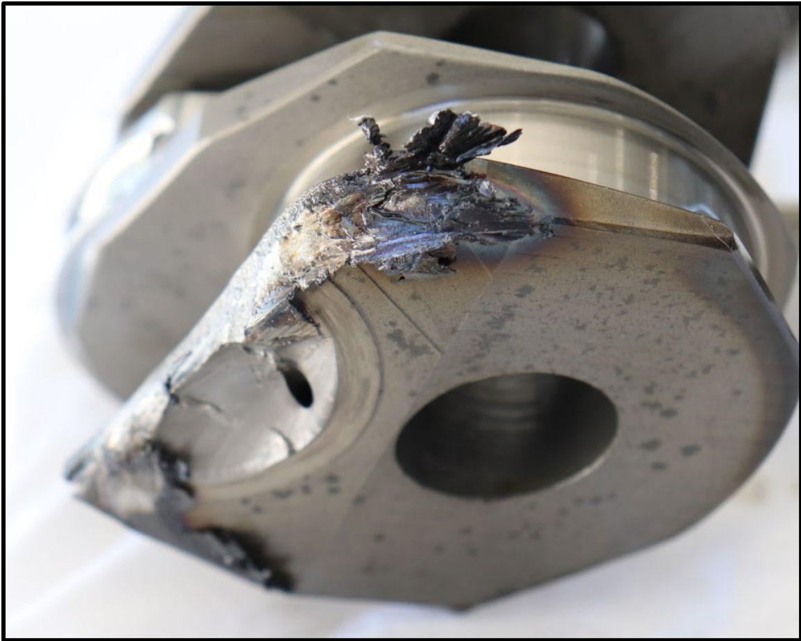
Figure 6: Crankshaft Fracture Surface
