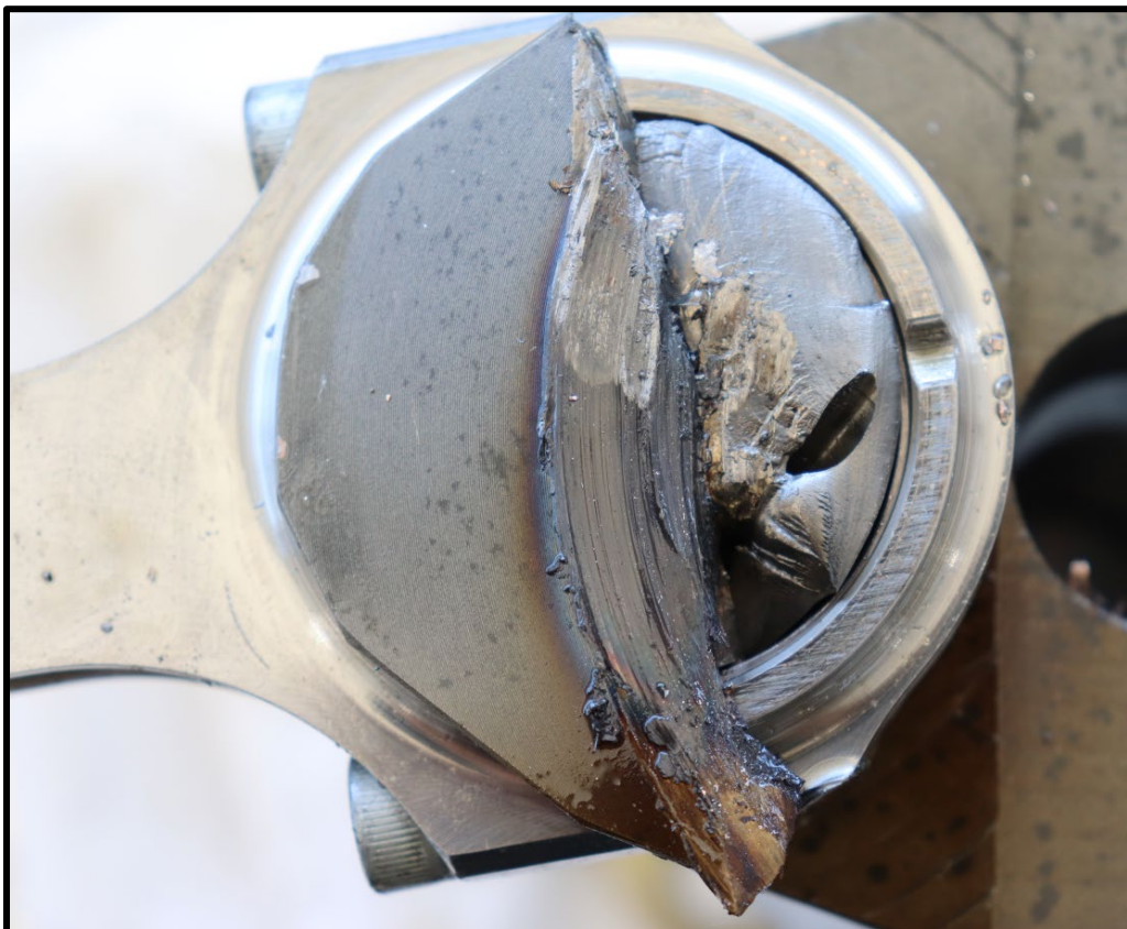
Figure 7: Crankshaft Fracture Surface (other side)
