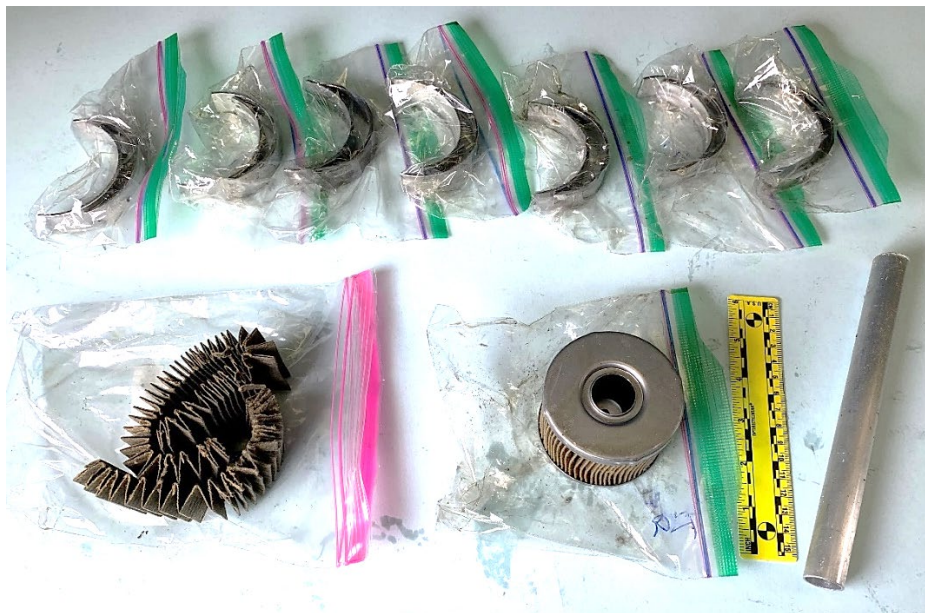
Figure 3. As-received parts consisting of seven pairs of main bearing halves; two filters (on left removed prior to accident and on right removed from airplane after the accident); and oil tube that was cut from the engine case to facilitate shipping.
