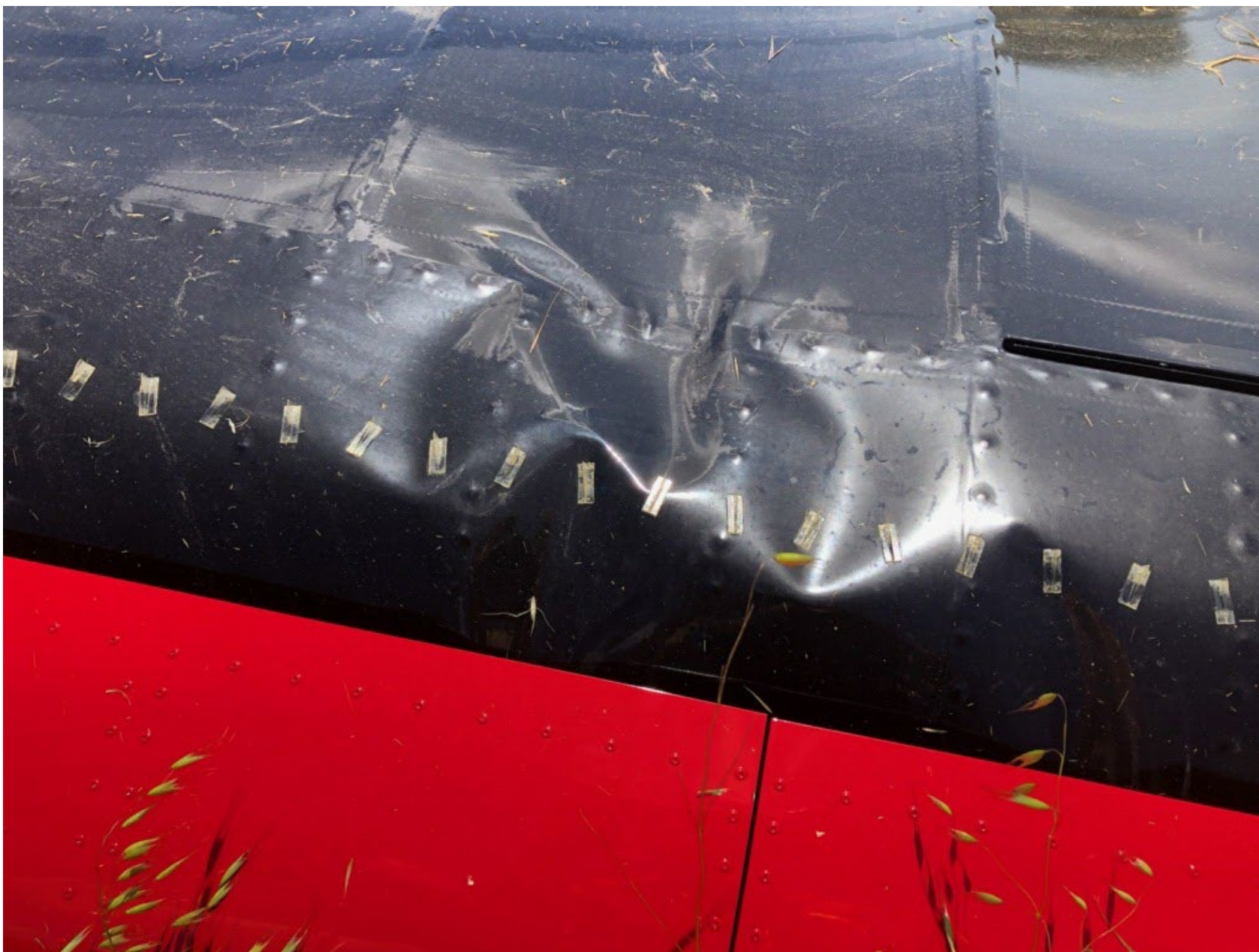
Photo 1 – View of substantial damage to left wing (provided by LEO)
