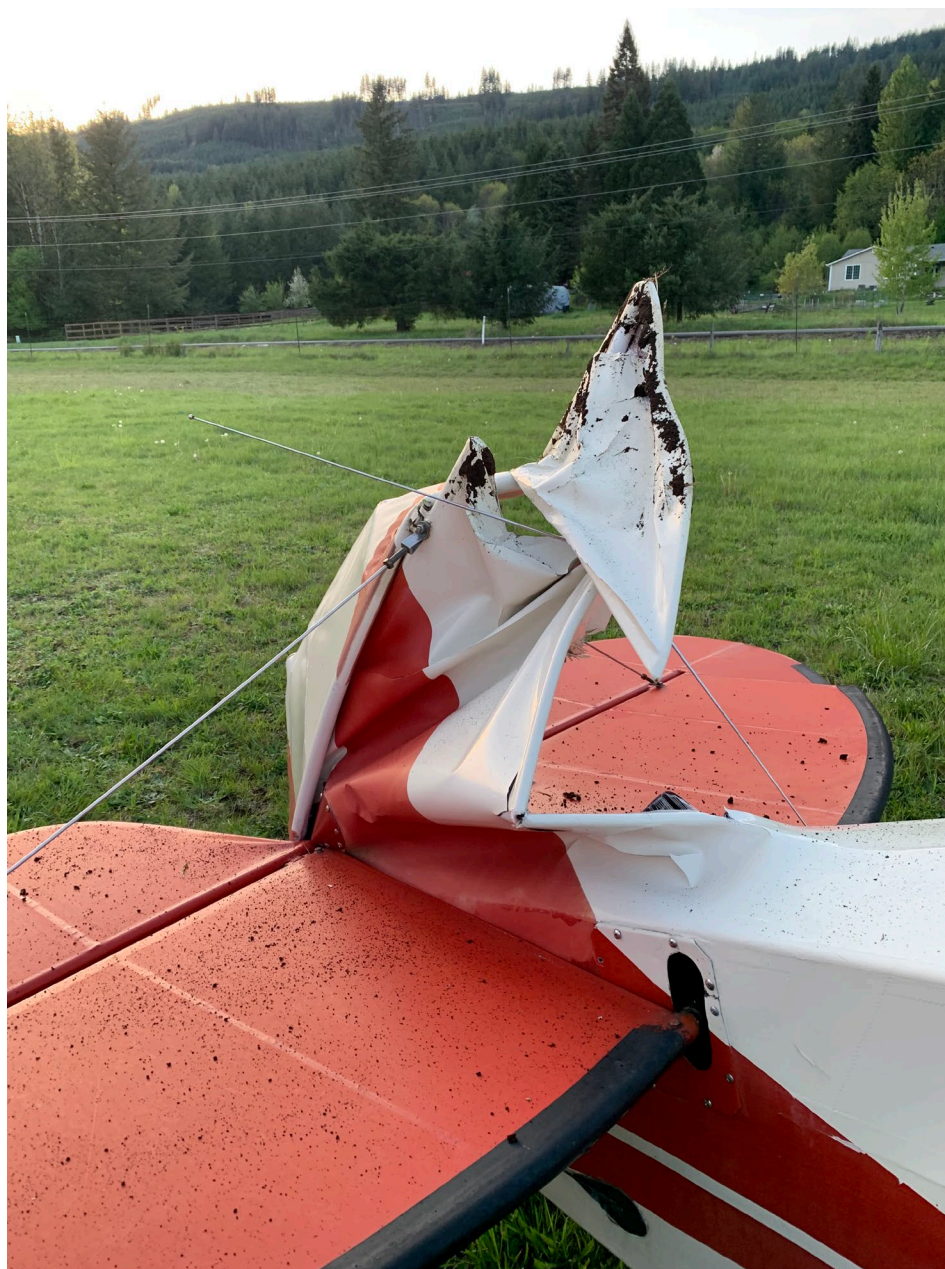
Photo 2 – (View of damage to vertical stabilizer and rudder (courtesy of pilot))
