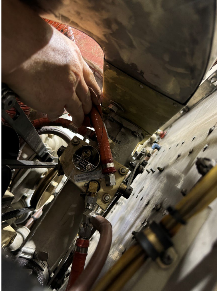
Figure 2: The fuel servo outlet line pulled away from the fuel servo.
