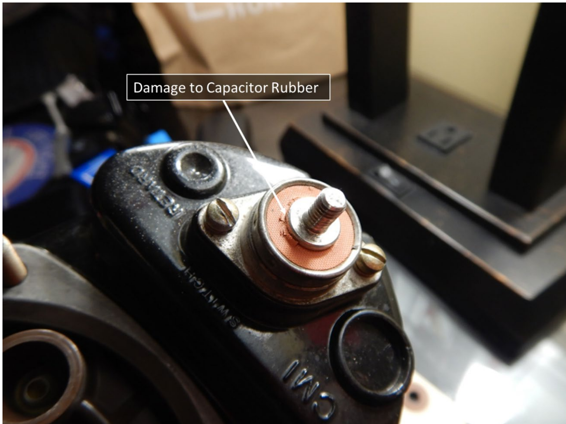
Figure 5. Torn rubber at the capacitor stud, F16HA264R
