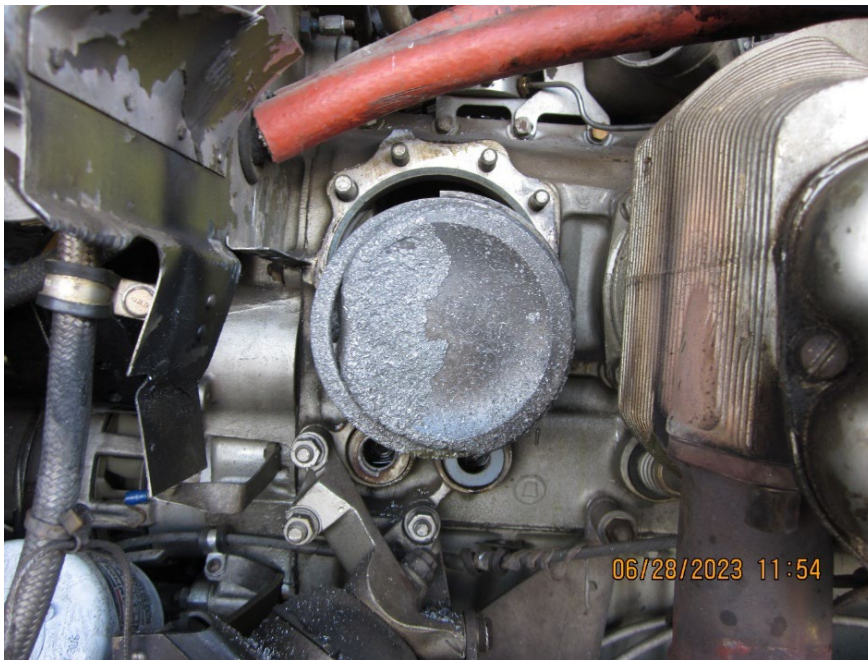
Figure 8: Front View of No. 1 Piston Face
