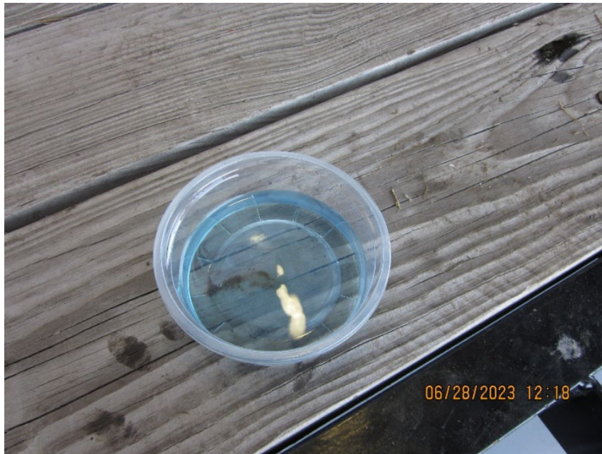
Figure 1: View of fuel from rear airframe fuel filter
