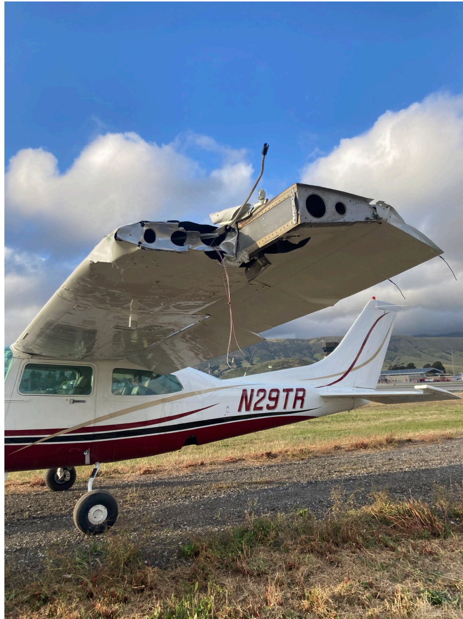
Photo 1 – View of substantial damage to left wing (courtesy of pilot)
