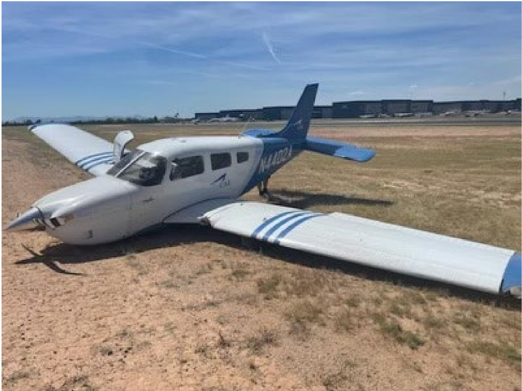
Photo 1 – Damage to Left Wing (Source: Instructor Pilot)
