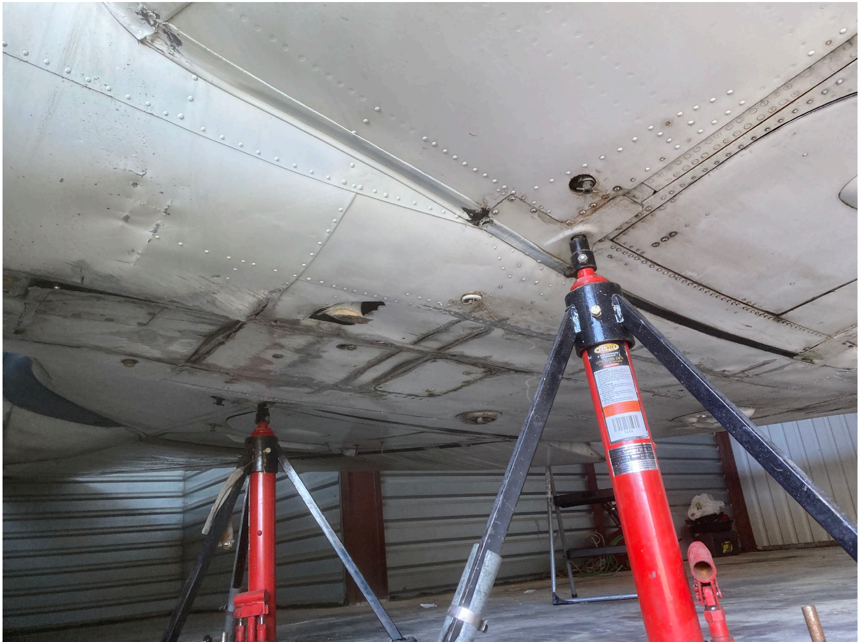
Photo 2 – Damage to the Lateral Wing Spar Carry-Through Structure (Courtesy of Pilot)
