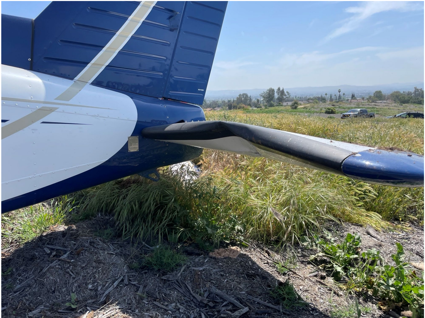
Photo 1 – View of damage to stabilator. (photo courtesy of LEO)
