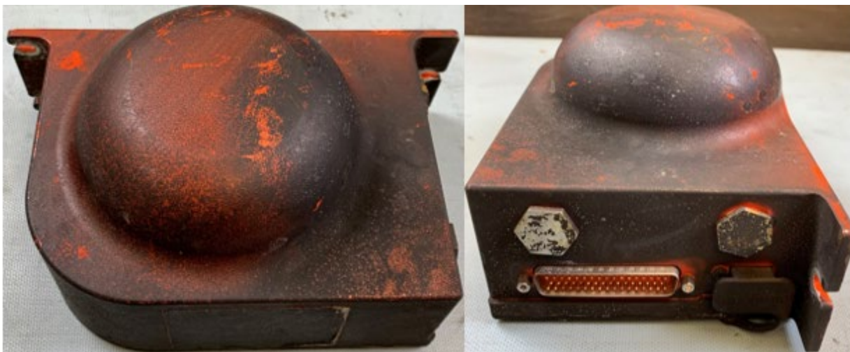
Figure 1. Top and side view of the L-3 LDR as received by the NTSB Vehicle Recorder Laboratory.
