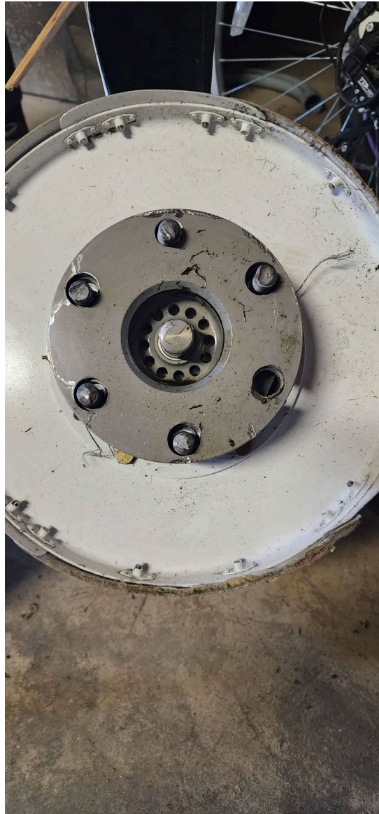
Photograph 5 - Propeller attachment bolts. (Courtesy of Morgan County Sherriff's Department.)
