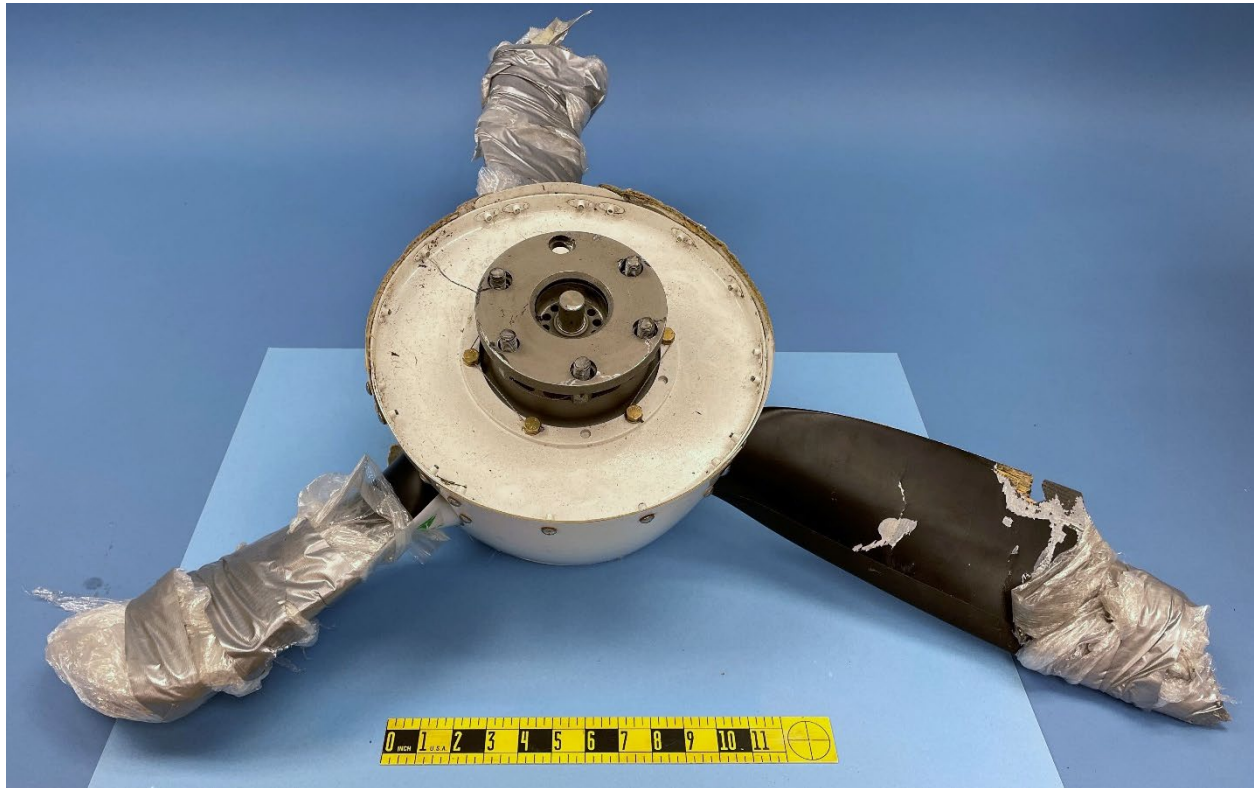
Figure 1. Separated propeller hub and blades, as received, viewed from the aft-facing side with fractured bolts and hub face.
