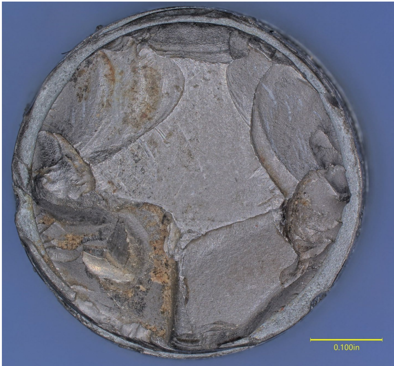
Figure 12. The fracture surface of Bolt 3.
