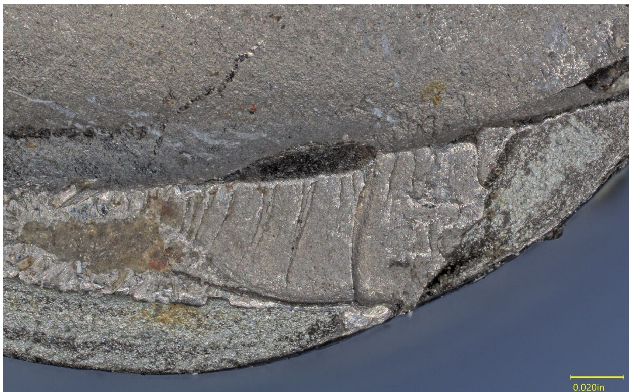
Figure 19. Closer view of secondary ratchet marks on the end of the Bolt 6 fracture surface.
