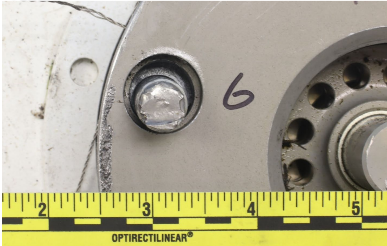
Figure 8. View of the fracture surface of the #6 bolt.
