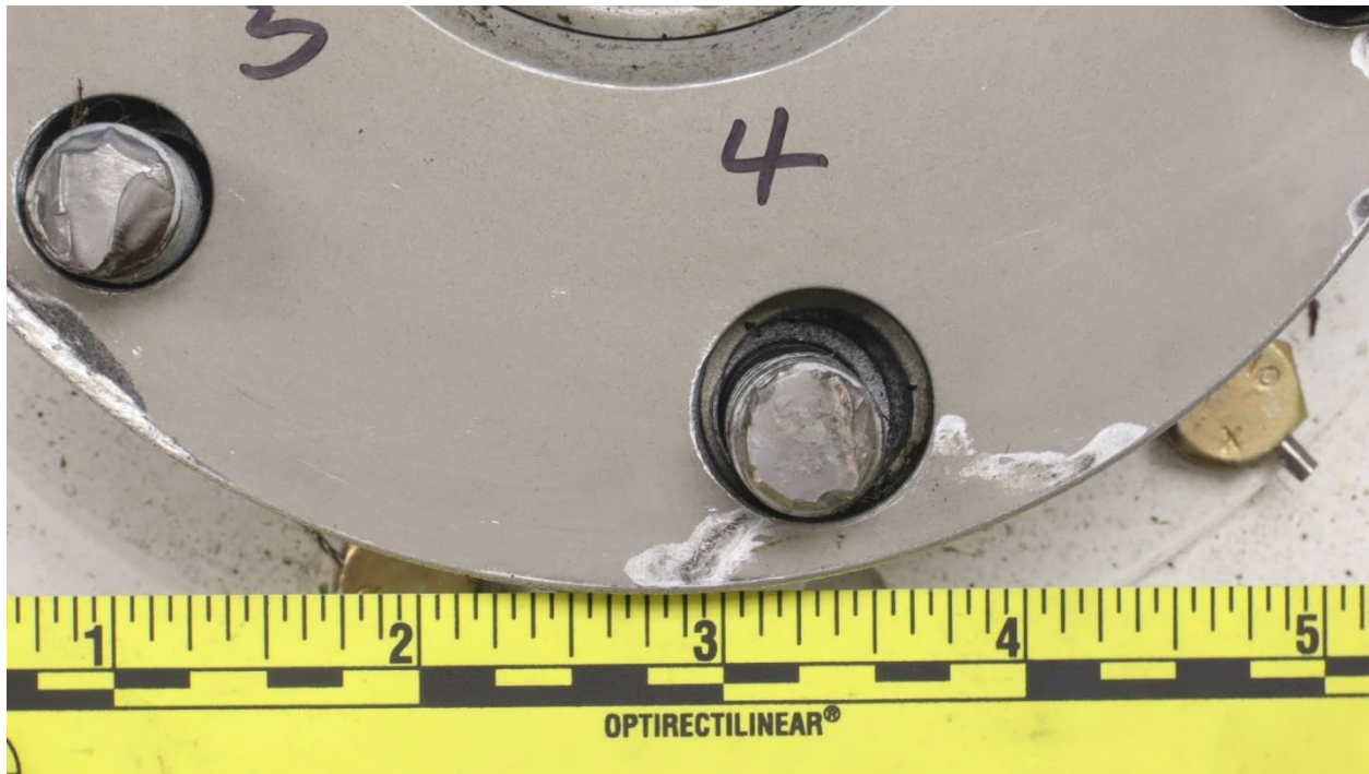
Figure 6. View of the fracture surface of the #4 bolt.
