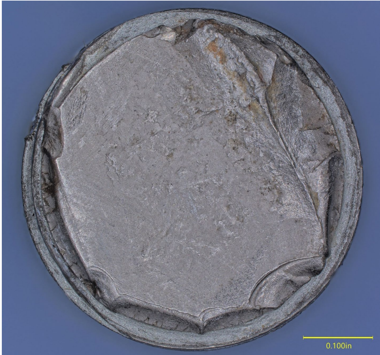
Figure 13. View of the Bolt 4 fracture surface.
