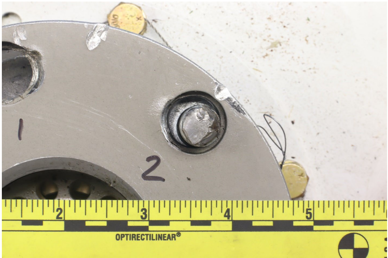
Figure 4. View of the fracture surface of the #2 bolt.
