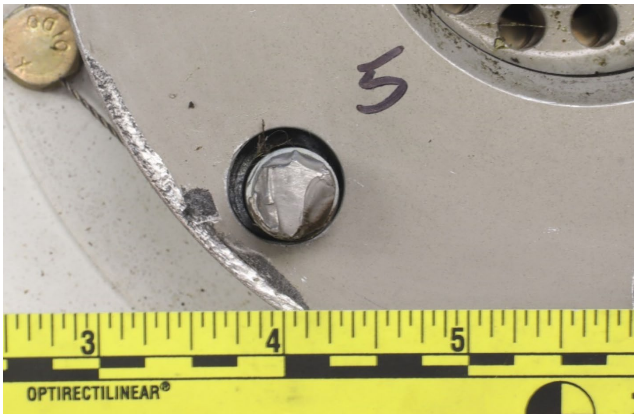
Figure 7. View of the fracture surface of the #5 bolt.
