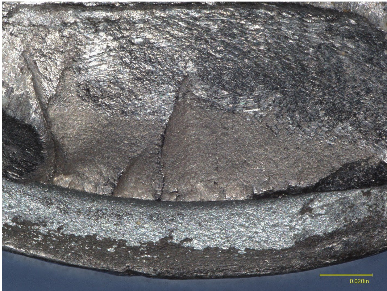
Figure 16. Closer view of ratchet marks near the edge of the Bolt 4 fracture surface.
