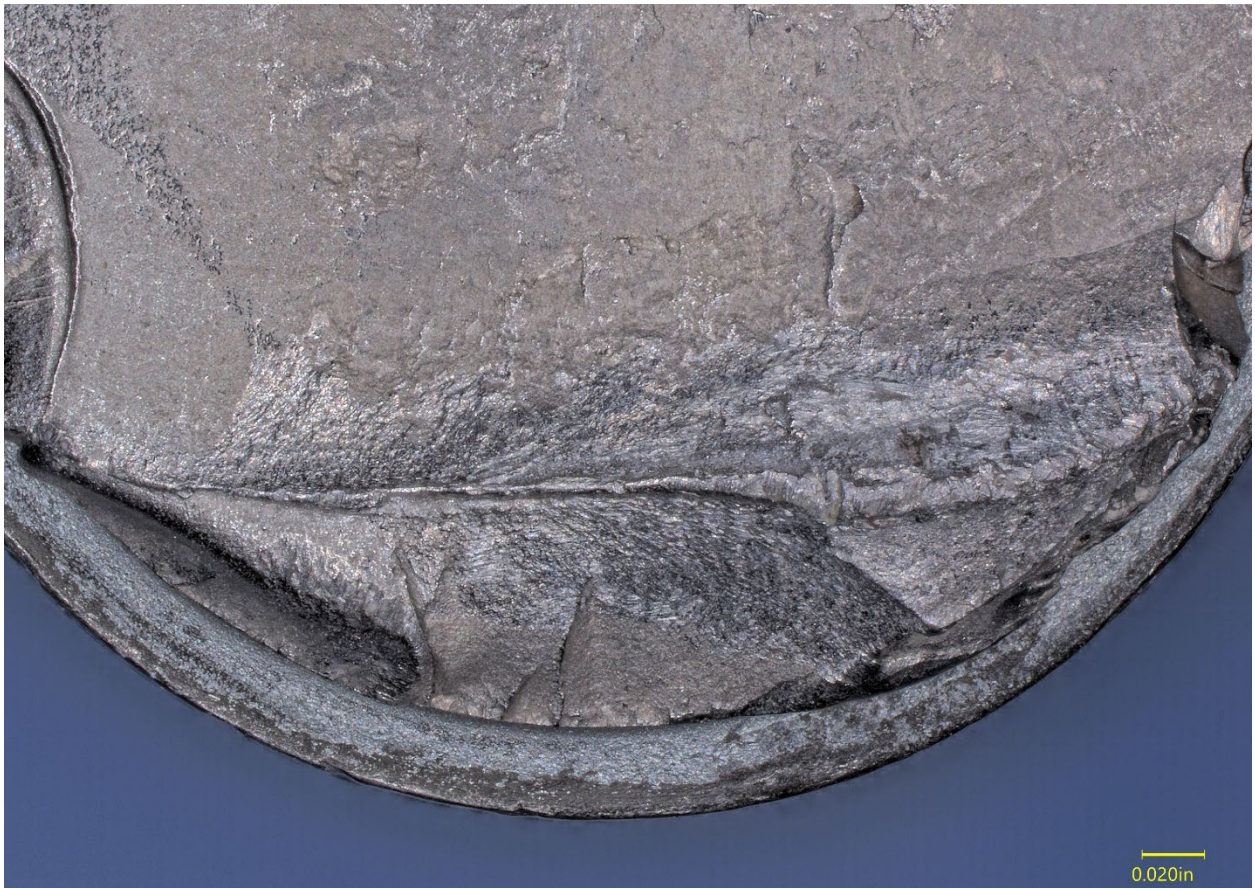
Figure 15. The upward facing ridge on the fracture surface of Bolt 4 (upper right in Figure 13).
