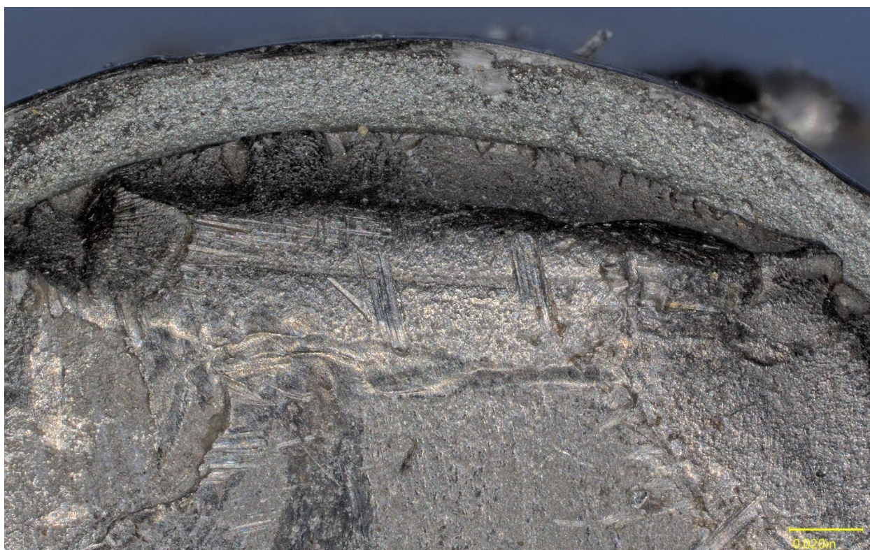
Figure 20. Smaller ratchet marks on the Bolt 6 fracture edge, along with smearing and gouge marks on the surface.
