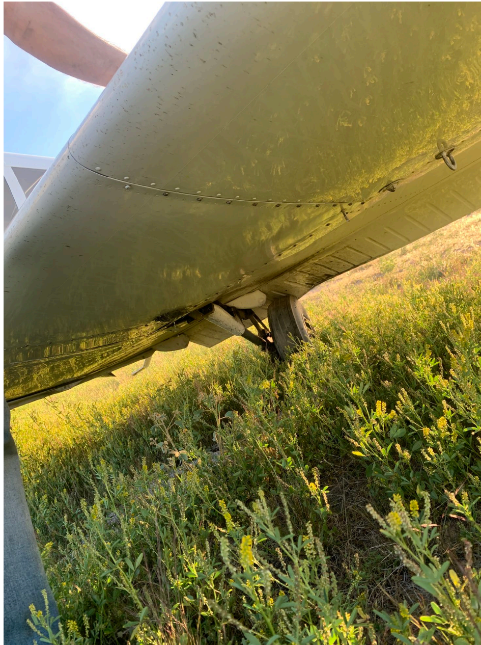
Photo 2 – View of Wing Damage (Courtesy of Pilot)
