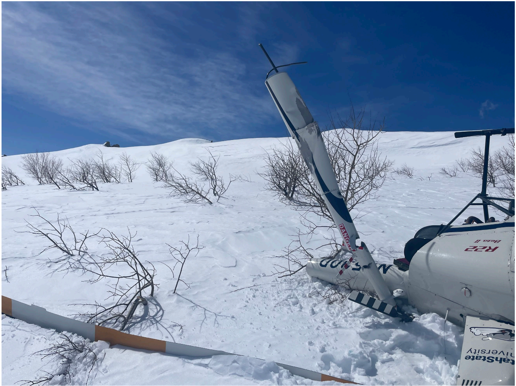
Photo 1 – View of substantial damage to tail boom (photo courtesy of pilot)
