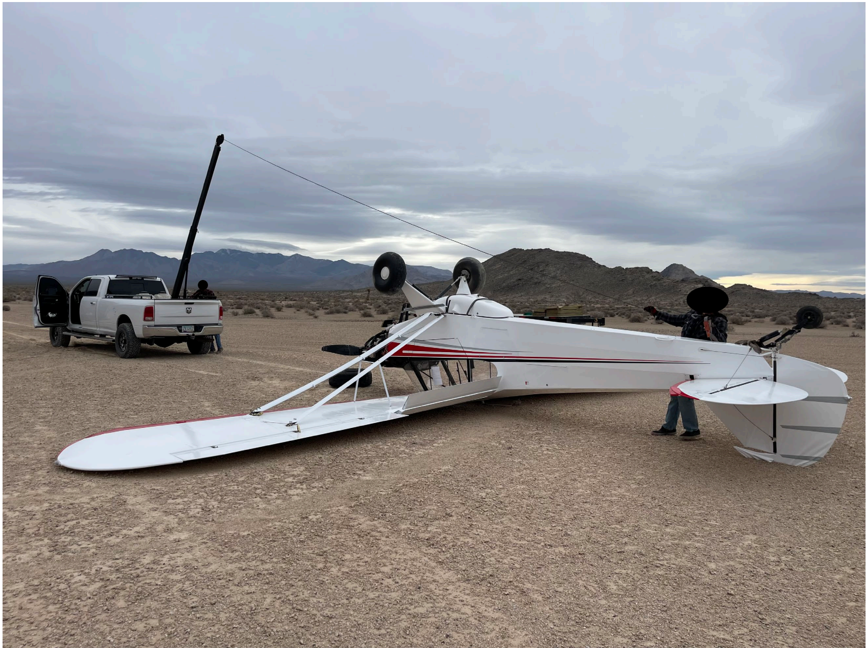
Photo 1 – View of substantial damage to vertical stabilizer and rudder (courtesy of pilot)
