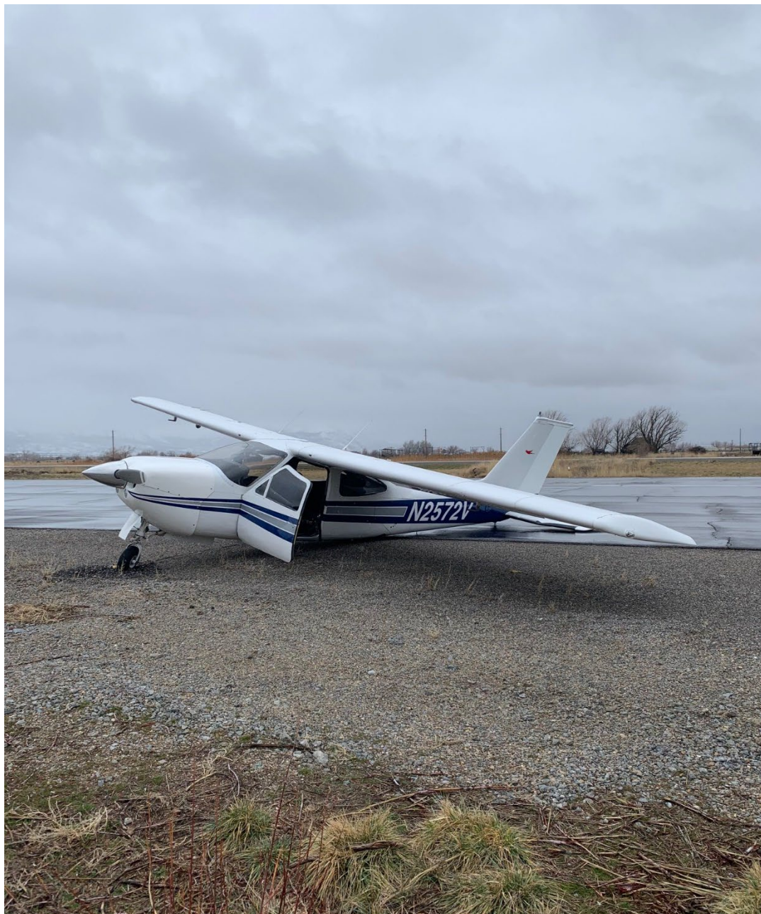
Photo 1 – View of nose landing gear extended, locked and main gear retracted (Courtesy of FAA)
