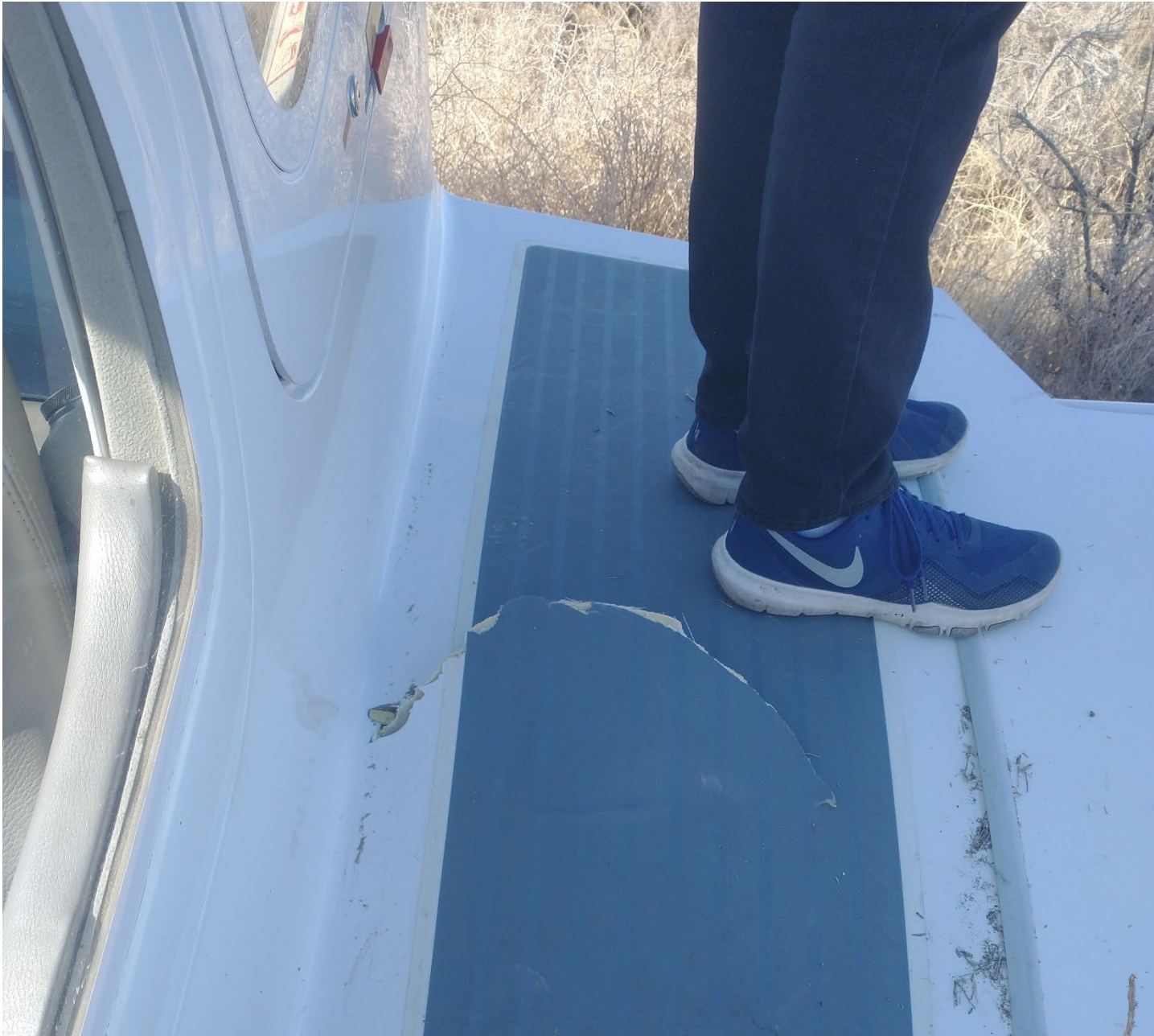
Photo 2 – View of damage to left wing root (courtesy of airport operations)
