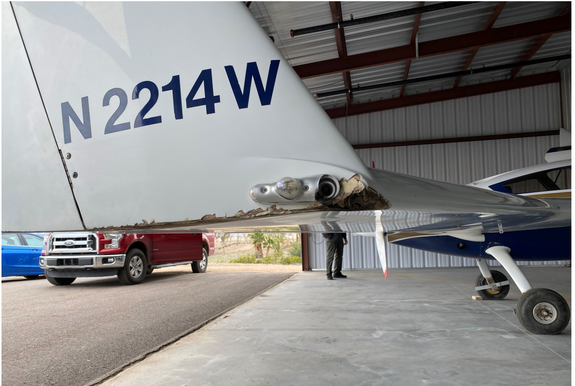
Photo 1 – View of damage to left wing tip (Courtesy of Owner)
