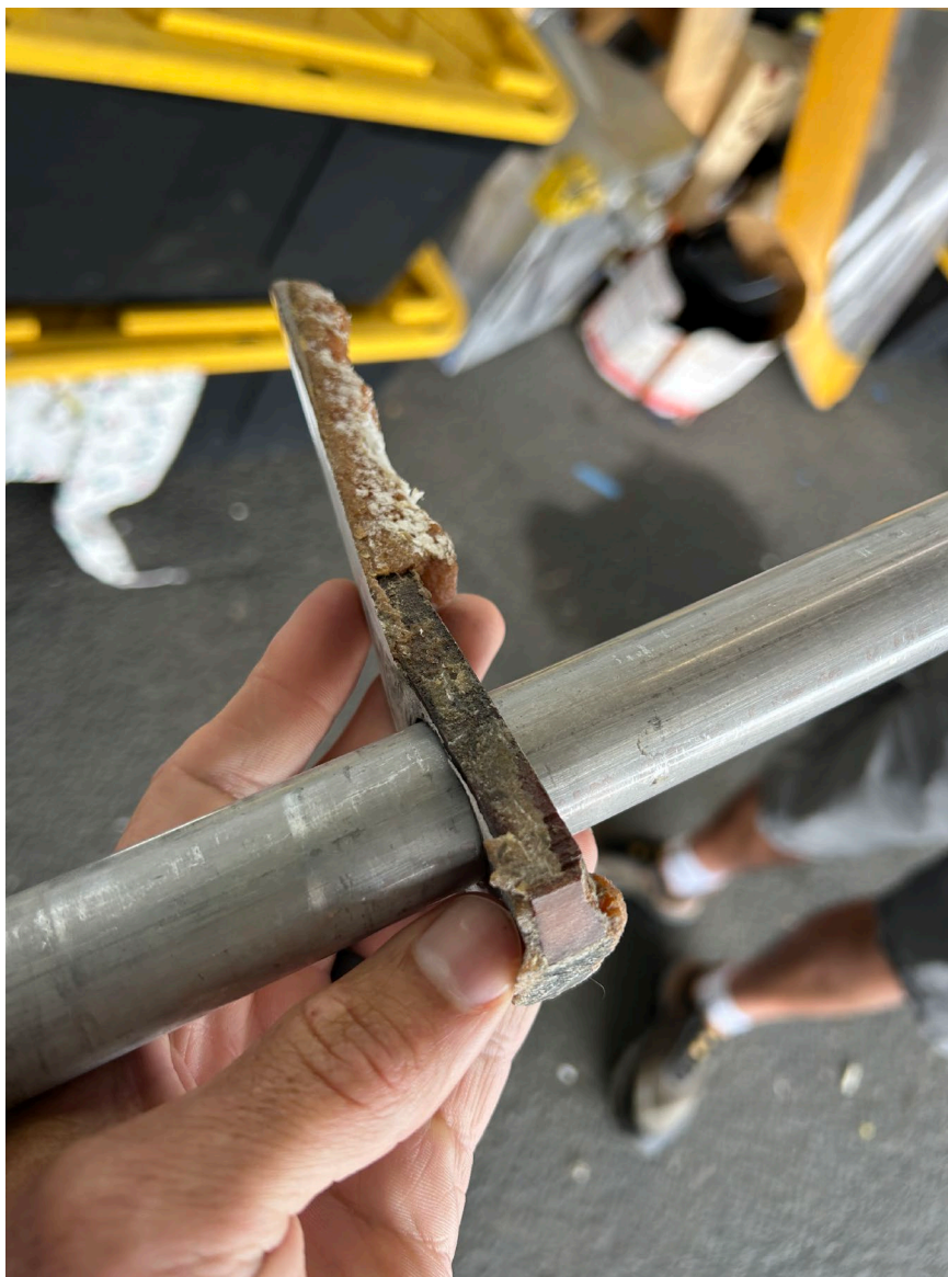
Photograph 6 - Outboard Trailing Edge Rib Lower Flange (Courtesy of Pilot)
