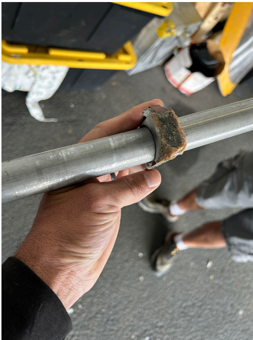
Photograph 5 - Outboard Trailing Edge Rib Forward Flange (Courtesy of Pilot)
