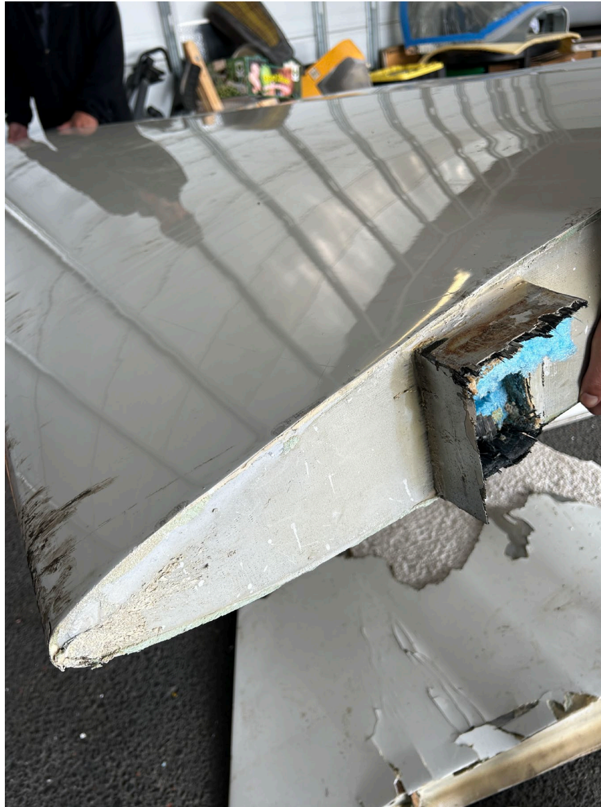
Photograph 7 - Left Wing Main Spar Separation (Courtesy of Pilot)
