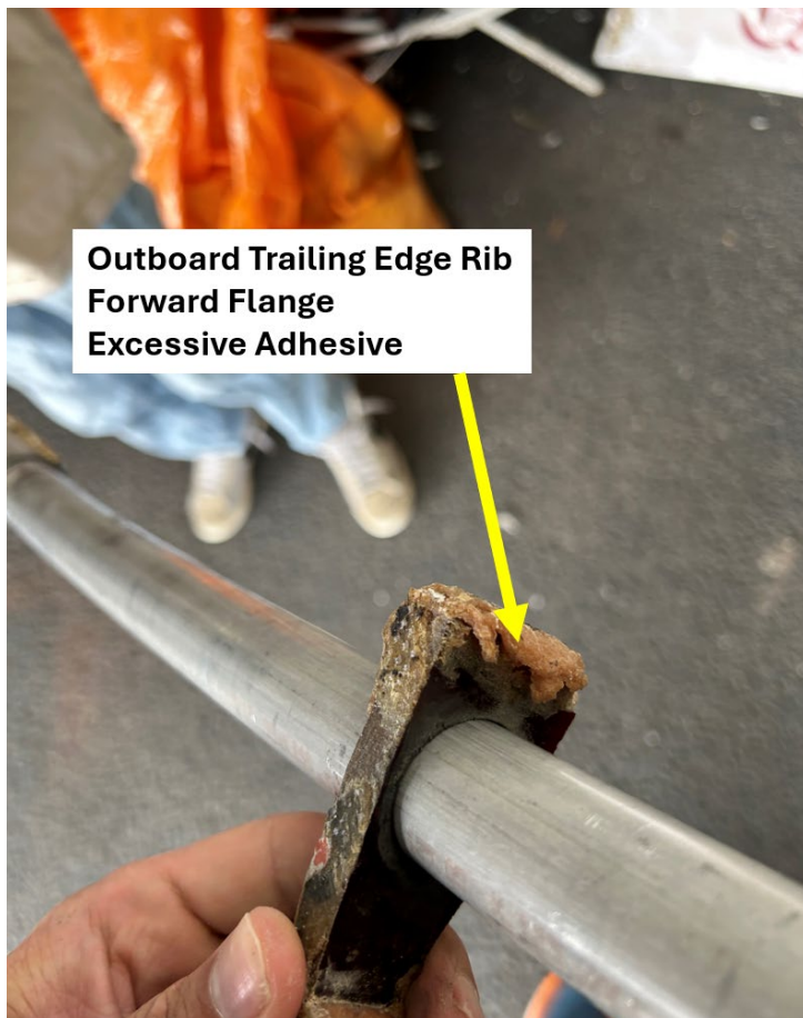
Figure 7 - Outboard Trailing Edge Rib Forward Flange (Courtesy of Pilot)
