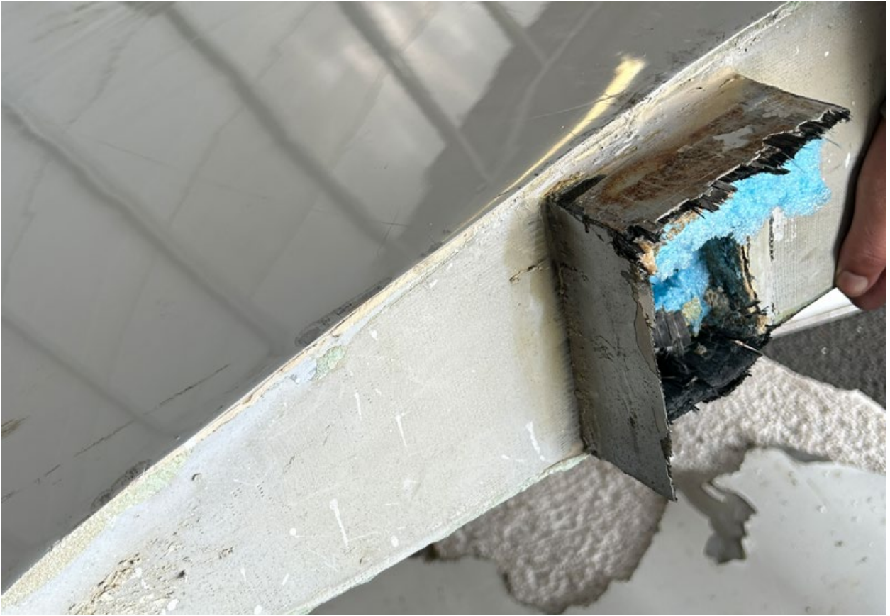
Figure 8 - Main Left Wing Spar Separation (Courtesy of Pilot)
