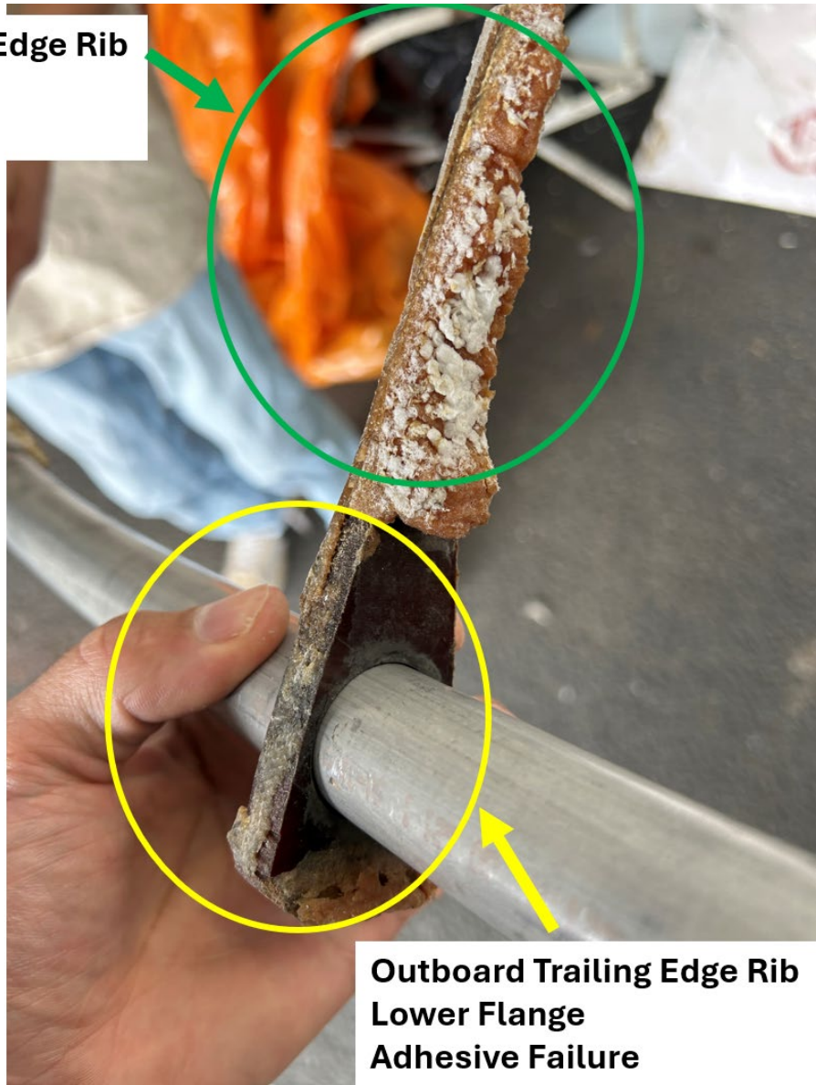
Figure 5 - Outboard Trailing Edge Rib Lower Flange (Courtesy of Pilot)
