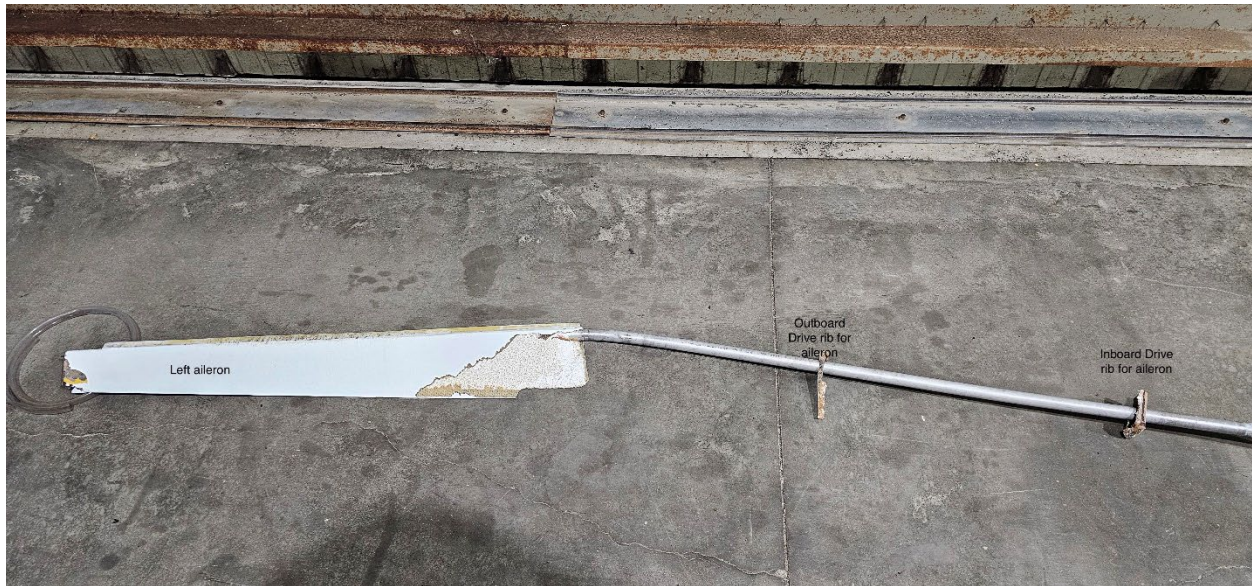
Figure 1 - Left Aileron and Torque Tube (Courtesy of Pilot)
