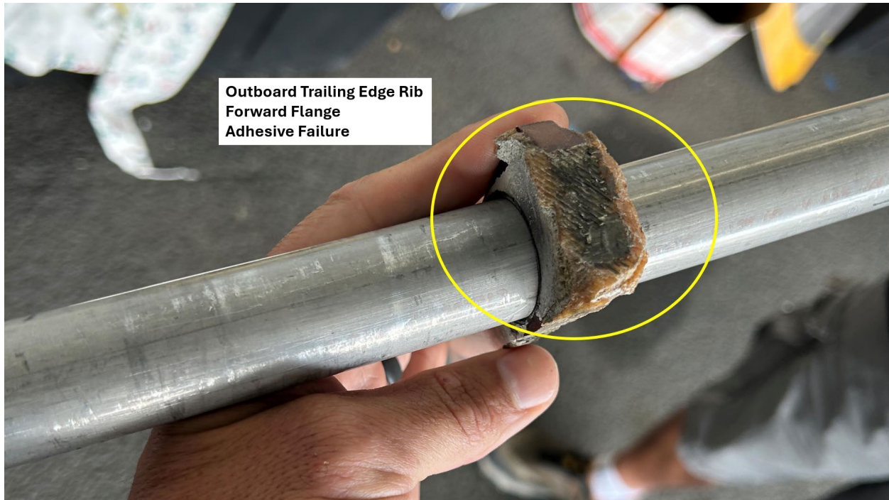
Figure 4 - Outboard Trailing Edge Rib Forward Flange (Courtesy of Pilot)
