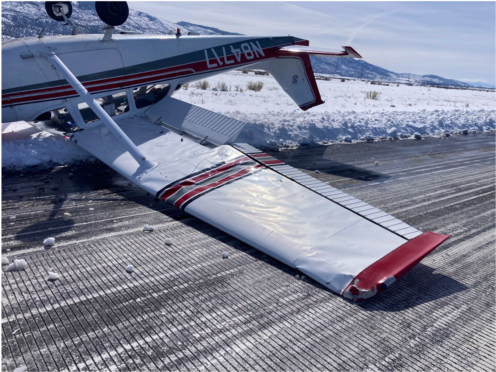
Photo 2 – View of substantial damage to right wing (courtesy of pilot)
