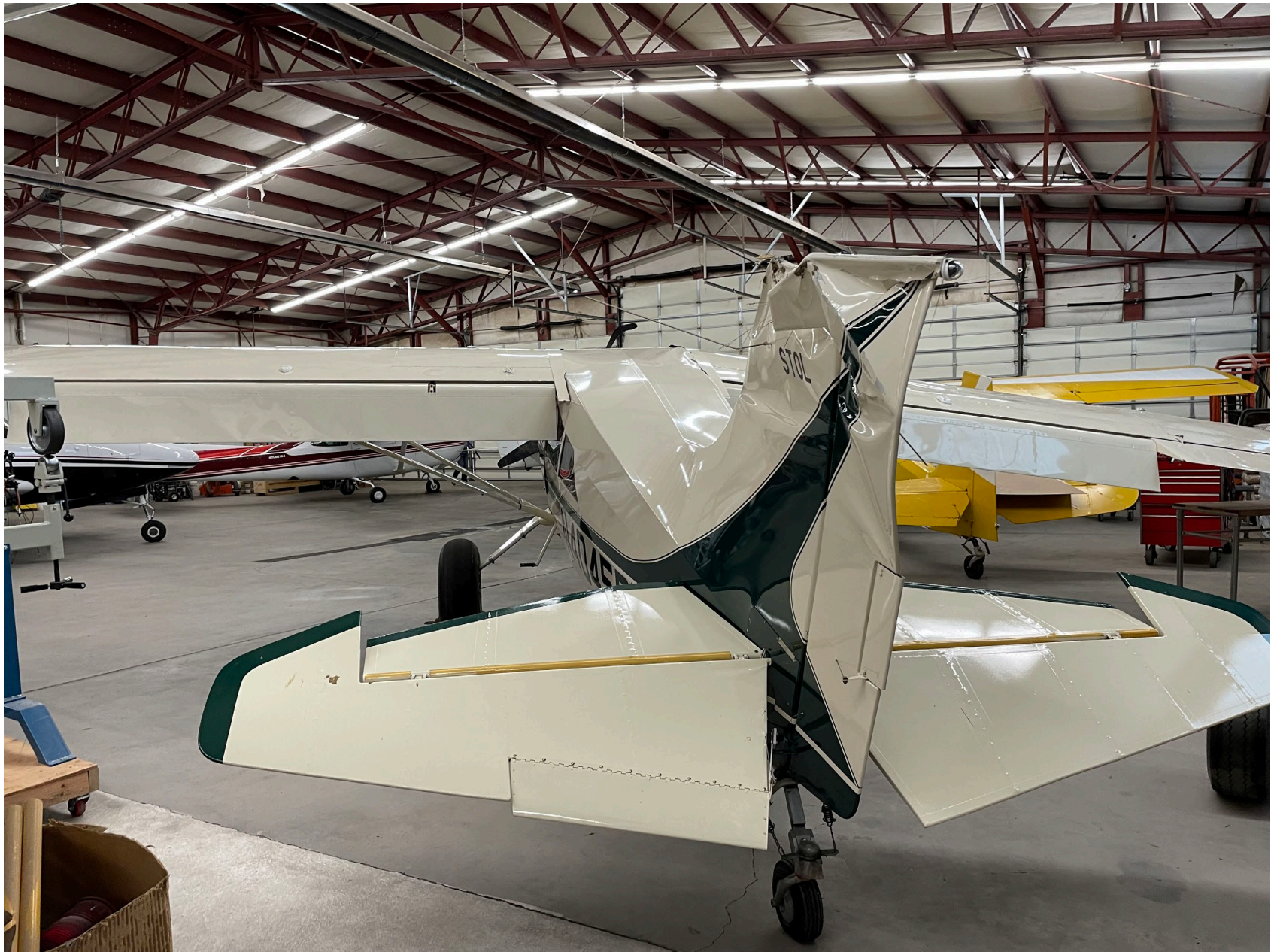
Photo 1 – View of substantial damage to vertical stabilizer and rudder
