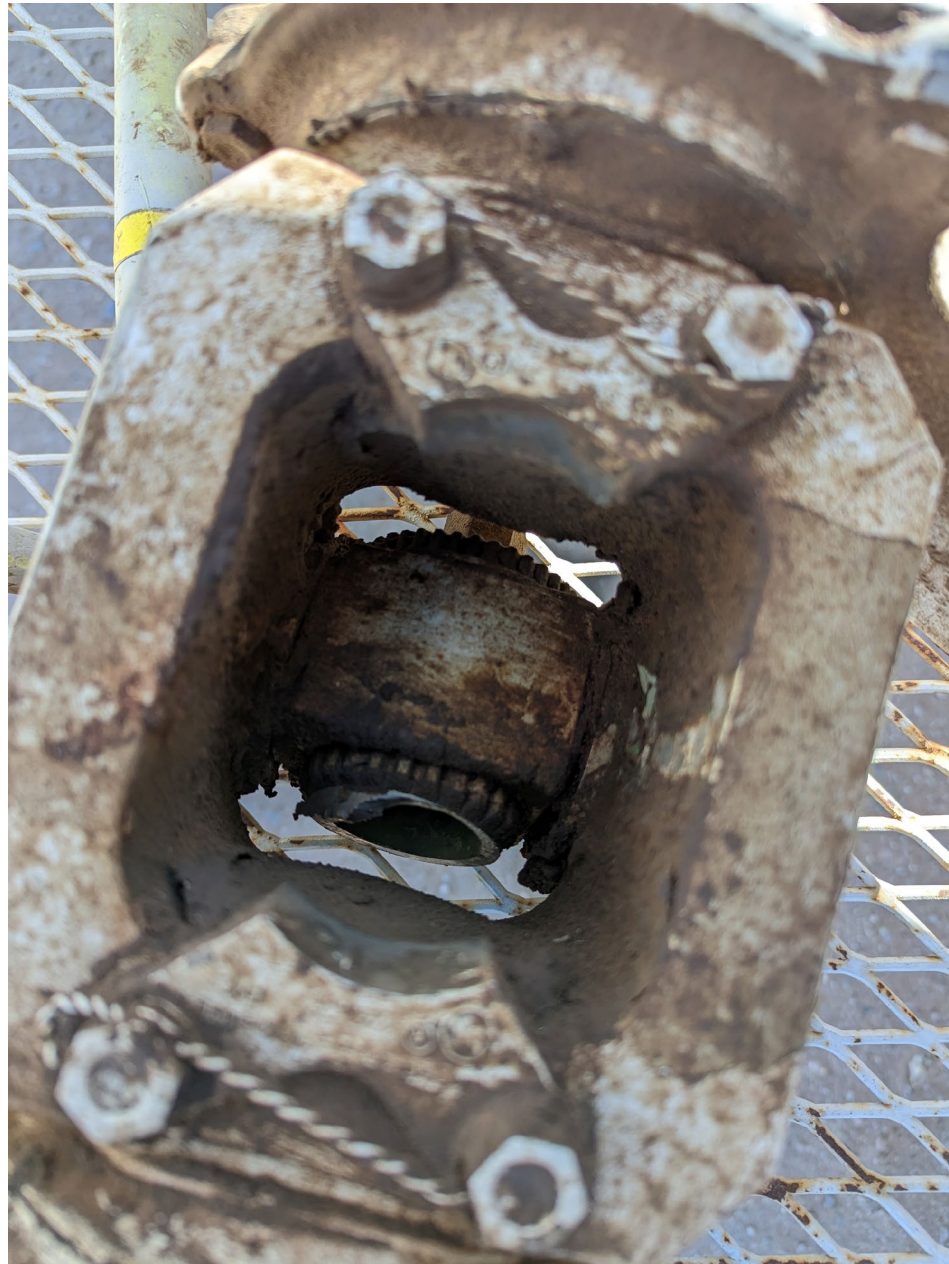
Photo 9 – View of rotor yoke at shear point
