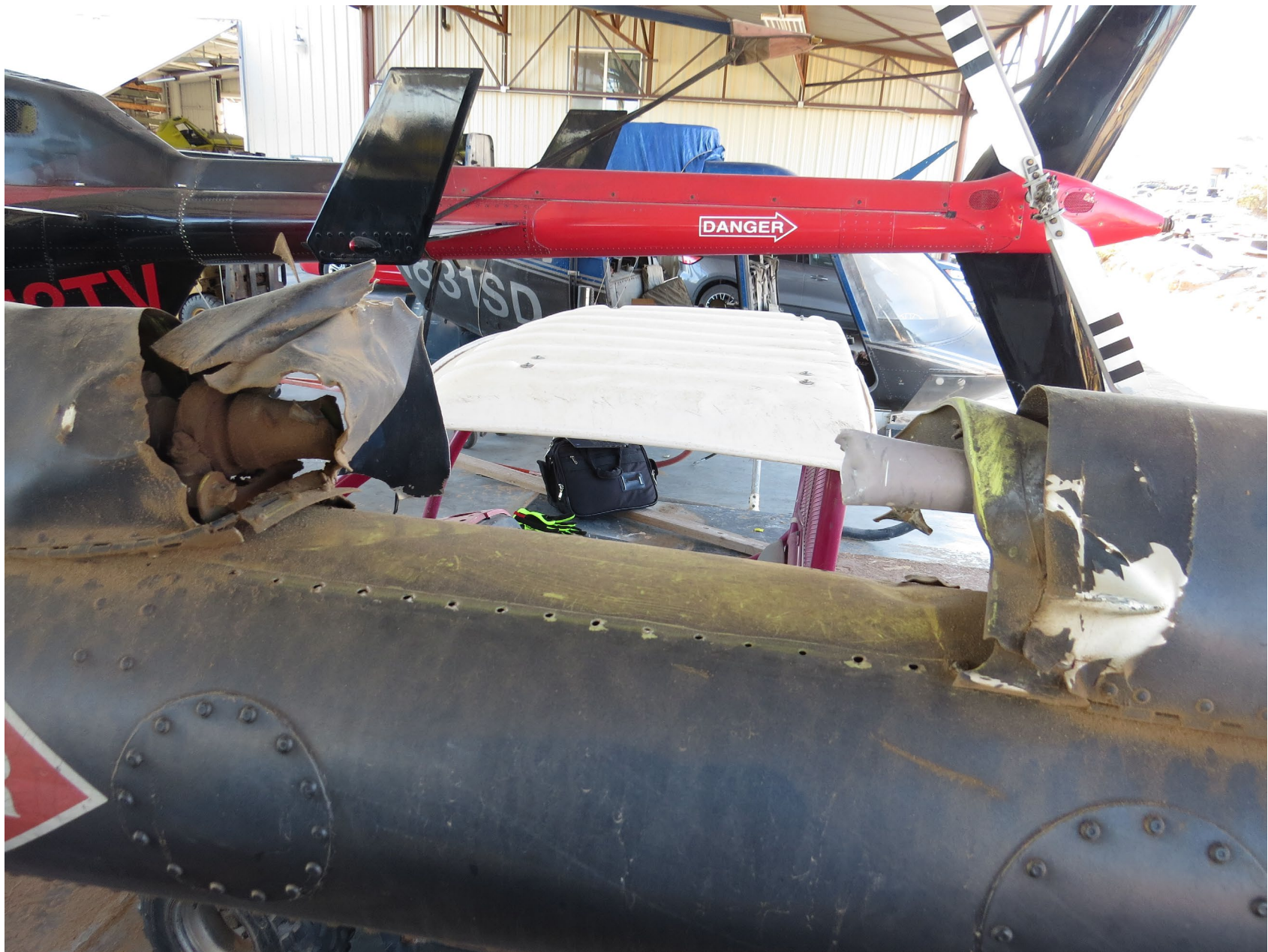
Photo 3 – View of tail rotor shaft rotor blade strike
