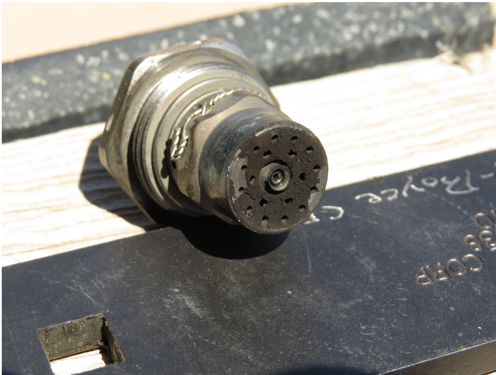
Photo 5 – Fuel nozzle removed at time of engine removal
