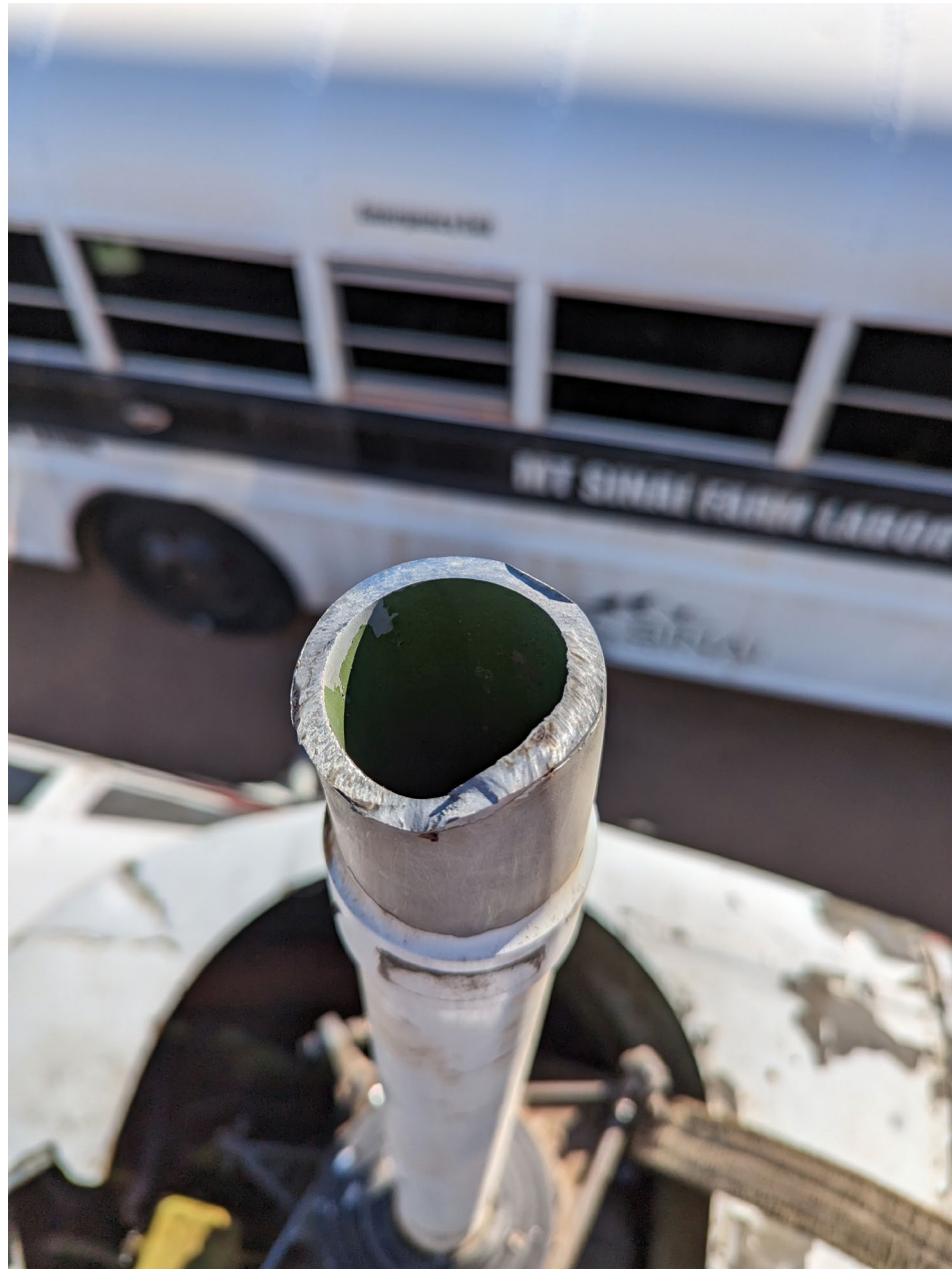
Photo 8 – View of rotor mast at shear point
