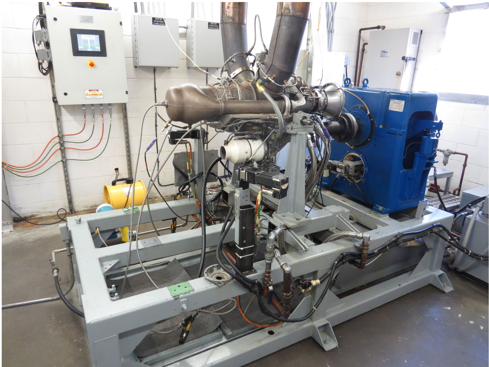
Photo 7 – Engine in test facility
