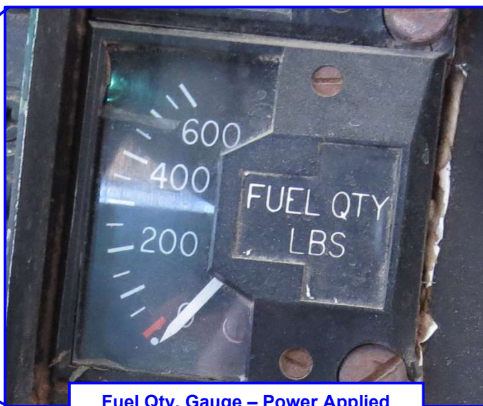
Fuel Qty. Gauge – Power Applied
