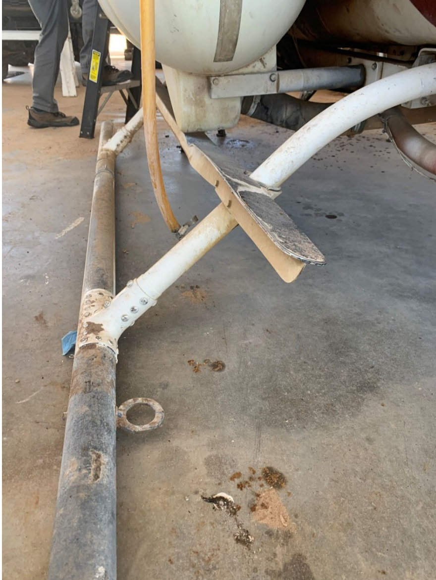
Figure 18. Right-side landing gear, showing downward dent to the upper step.
