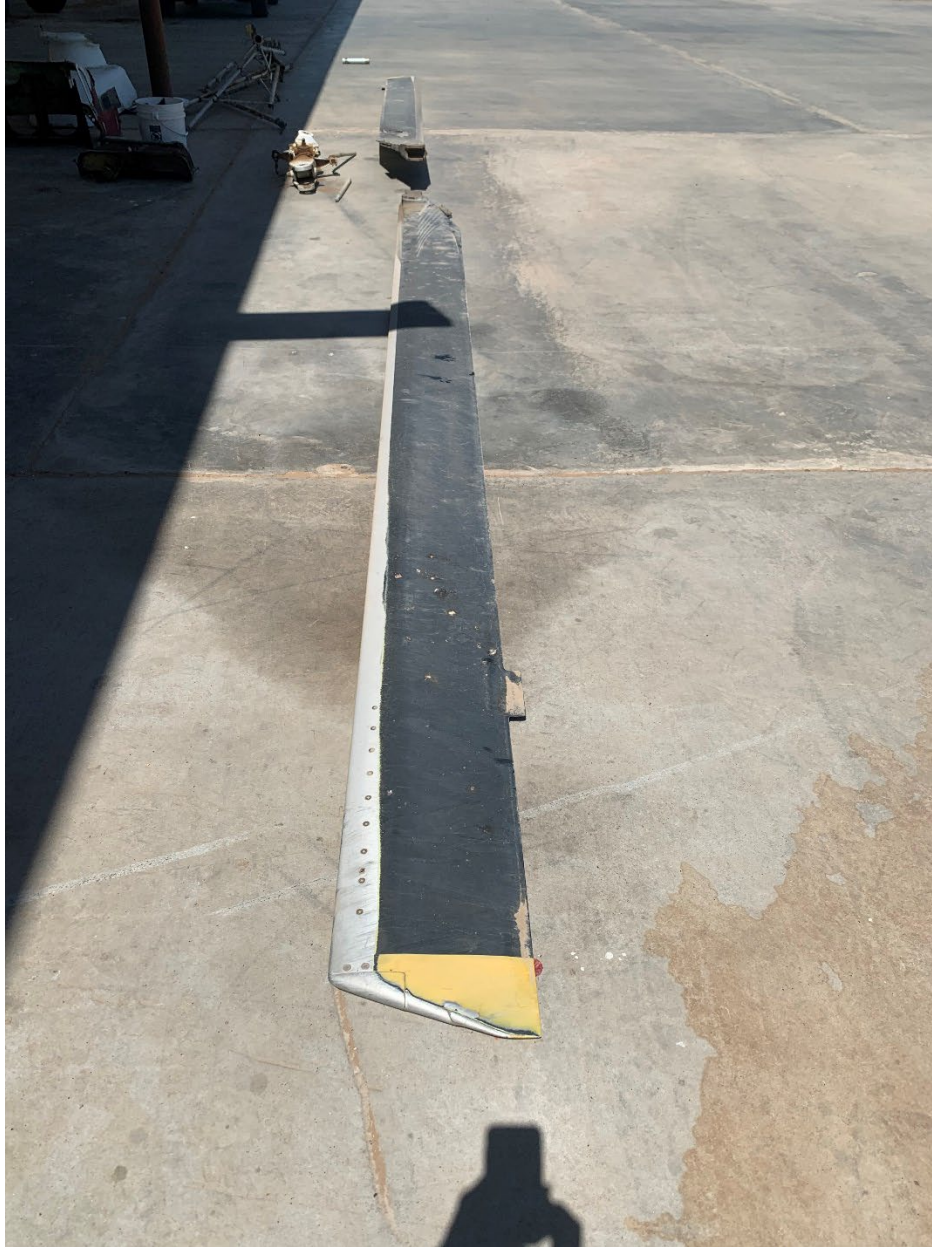
Figure 9. Blade CSFS-999, underside view. Note the damage at the tip.
