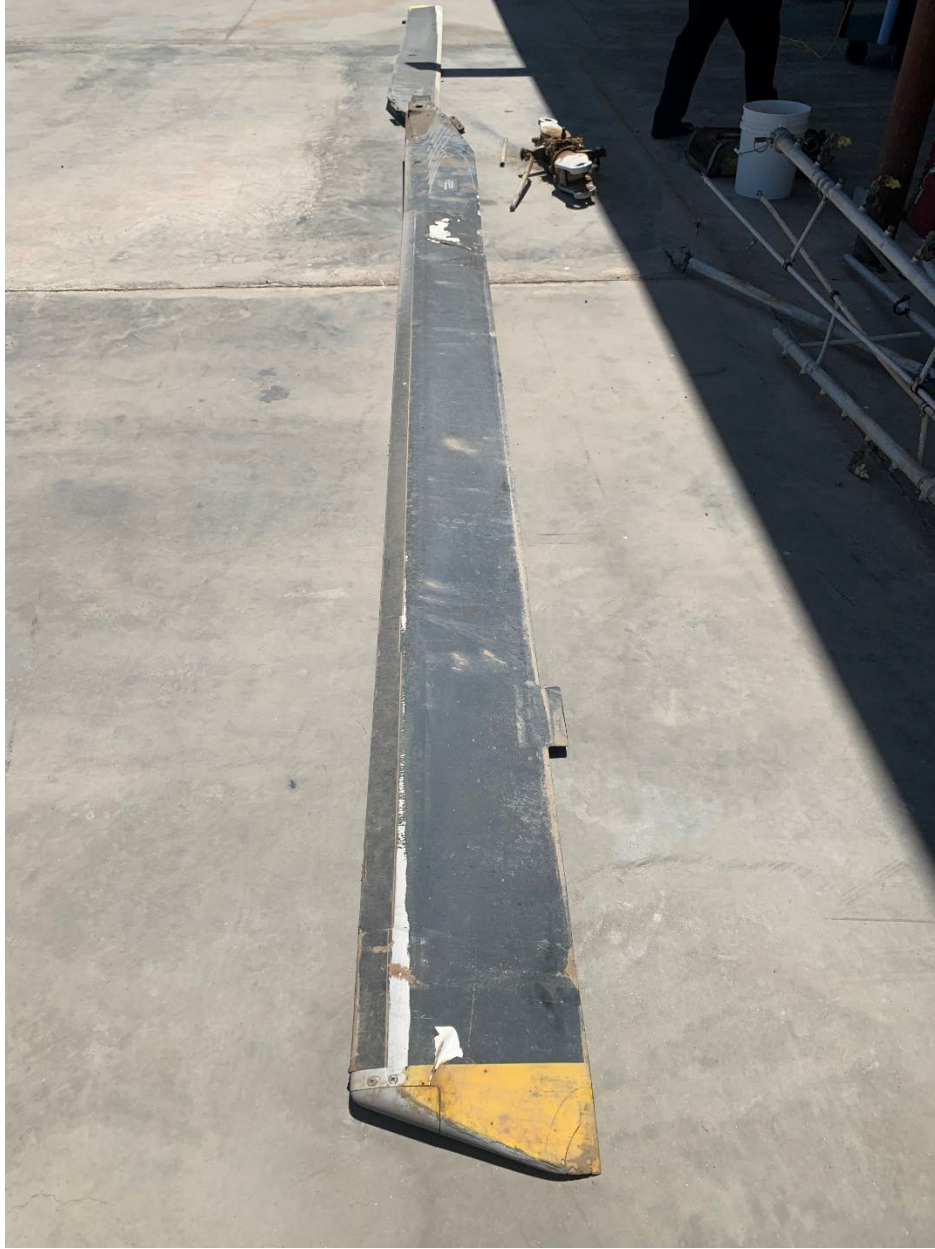
Figure 8. Blade T-FS-451 underside view. Note the damage near the root.
