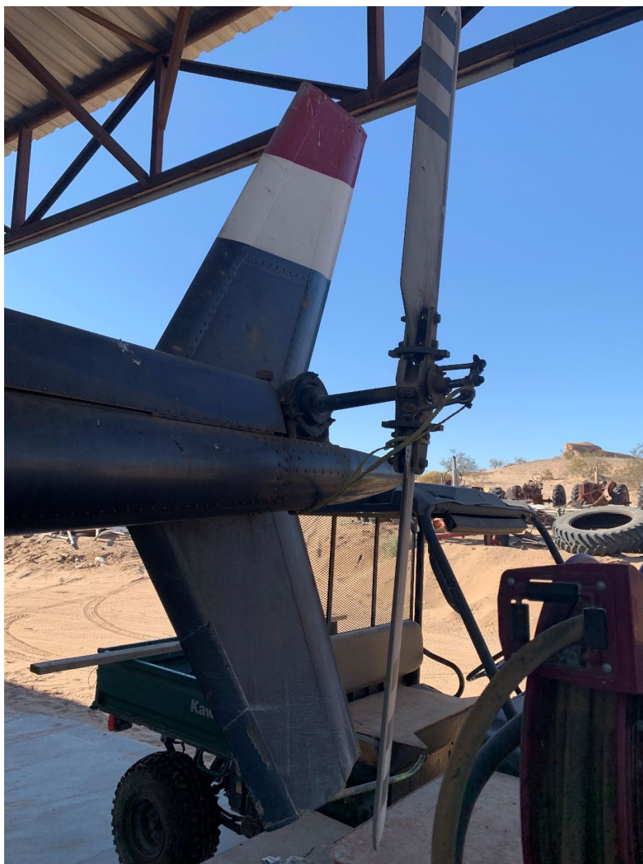
Figure 16. Tail rotor assembly and vertical stabilizer.
