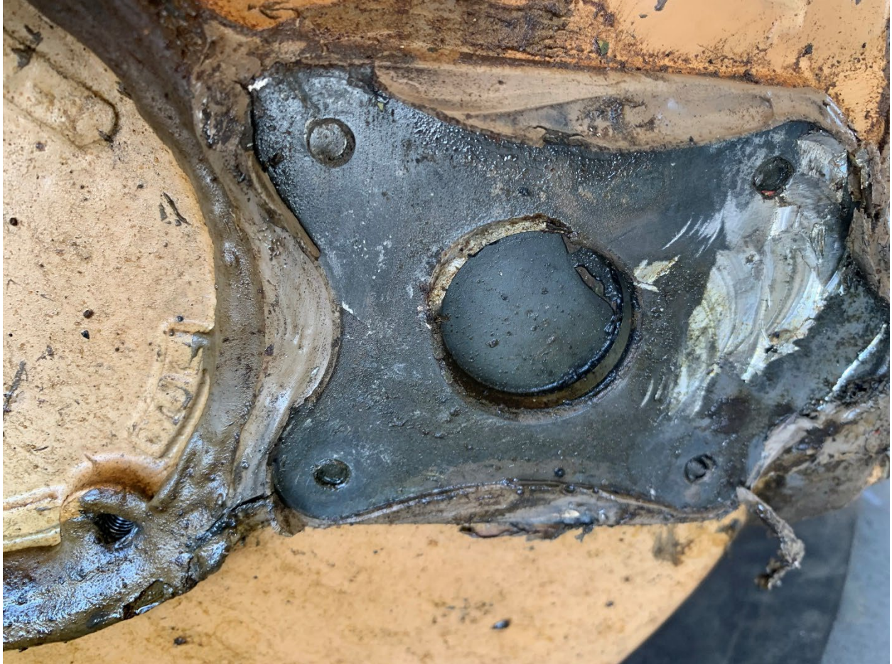
Figure 14. Lower transmission. Note the four sheared attachment studs.
