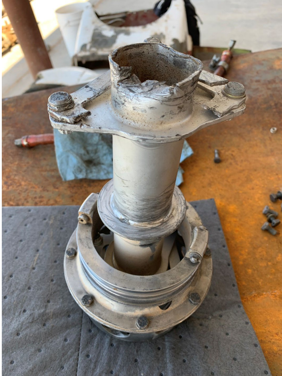
Figure 15. KAflex drive shaft. The damaged end attached to the transmission.
