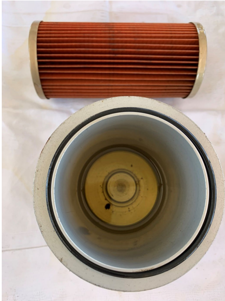
Figure 20. Residual fuel in deck-mounted fuel filter and filter element.
