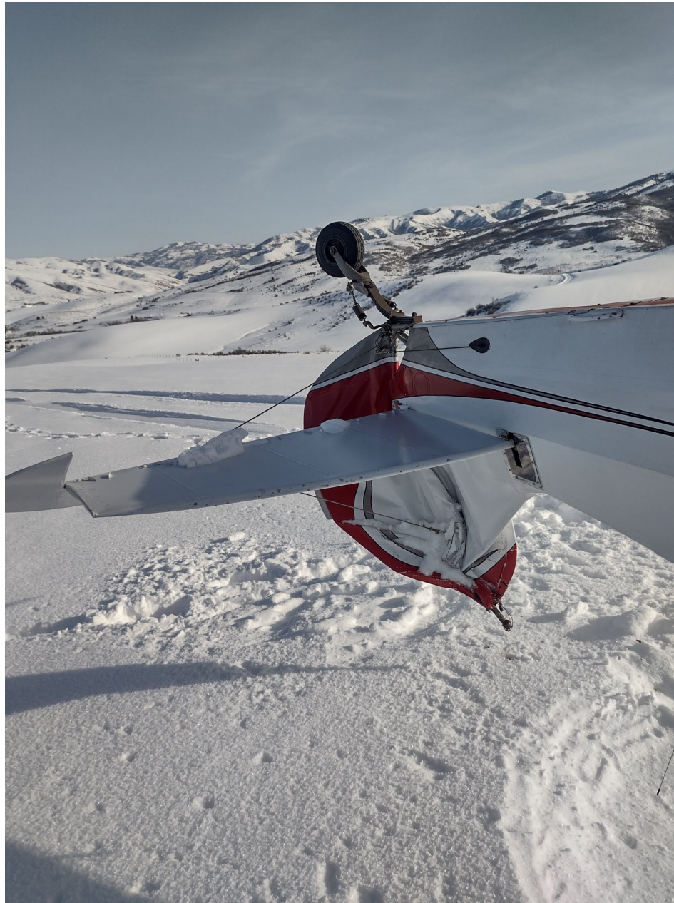
Photo 2 – View of Rudder and Vertical Stabilizer Damage
