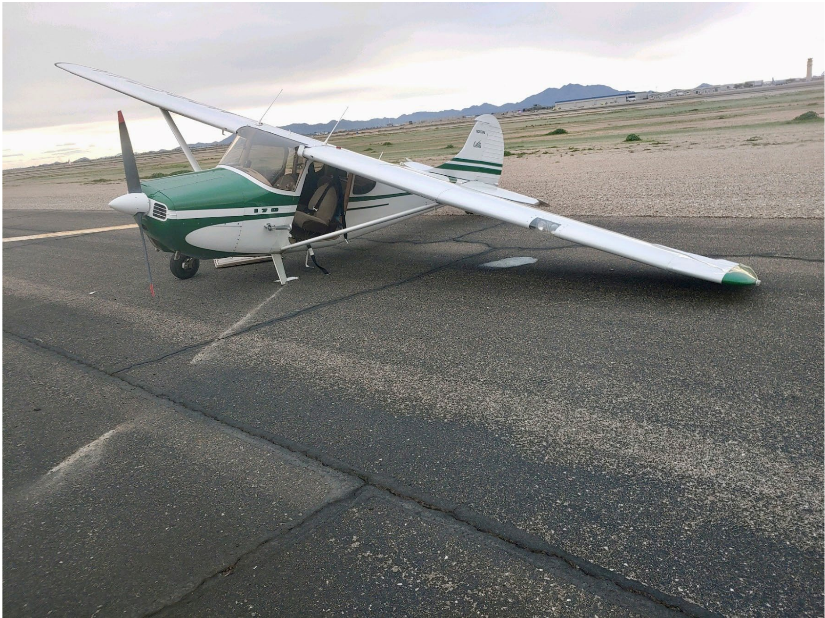
Photo 2 – View of damage to left wing and fracture separated landing gear leg (photo courtesy of pilot)
