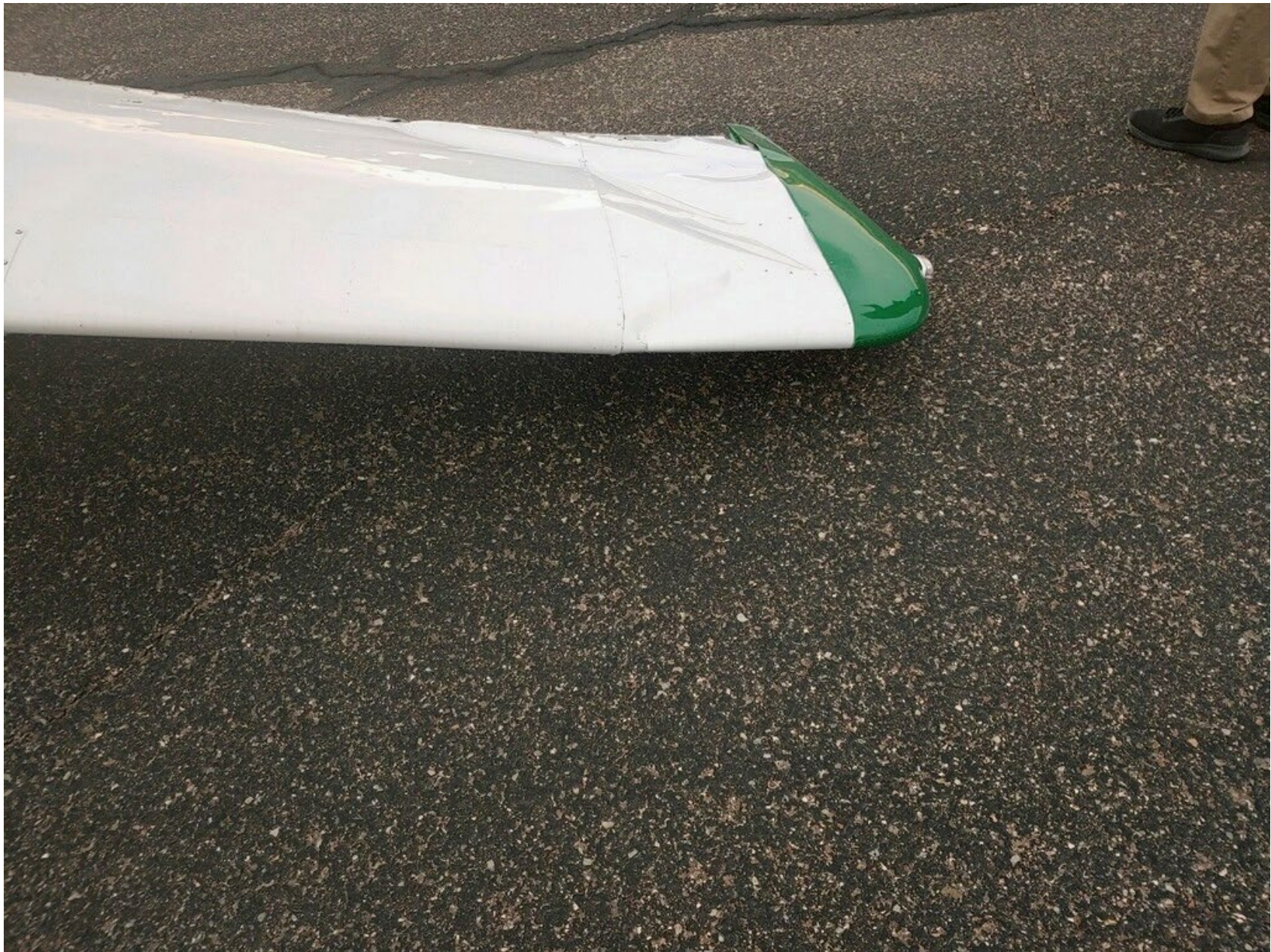
Photo 1 – View of substantial damage to left wing (photo courtesy of pilot)
