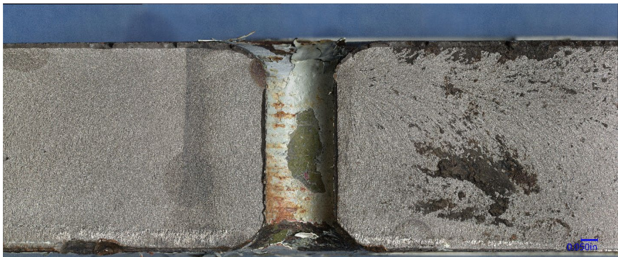
Figure 3. Montage of the cleaned fracture surface near the centerline clip bore.
