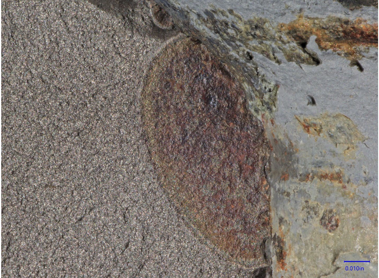
Figure 6. The largest thumbnail crack in the upper left of Figure 5 , showing crack arrest marks.
