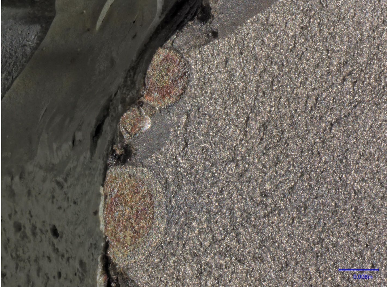
Figure 7. View of the smaller thumbnail cracks in the upper right of Figure 5 , showing crack arrest marks.
