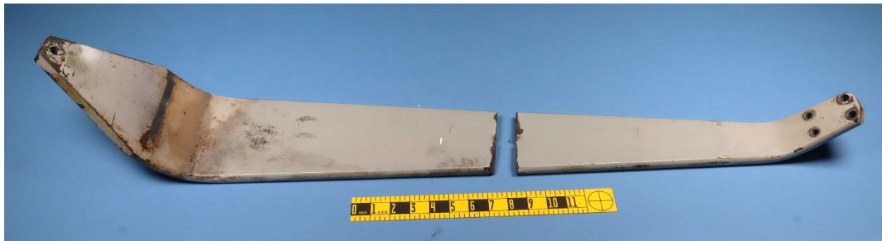
Figure 1. View of the landing gear leg pieces, as received.
