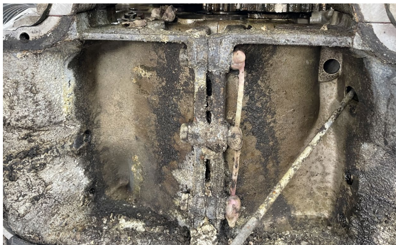
Figure 2: Upper section of oil sump with saltwater corrosion
