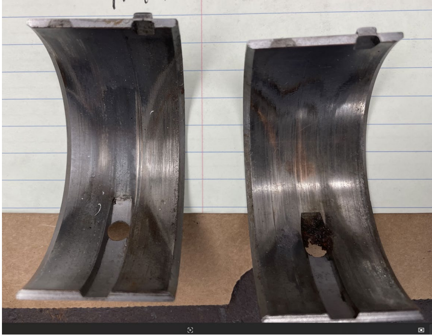
Figure 4: Center bearing with heat damage and rotational scoring
