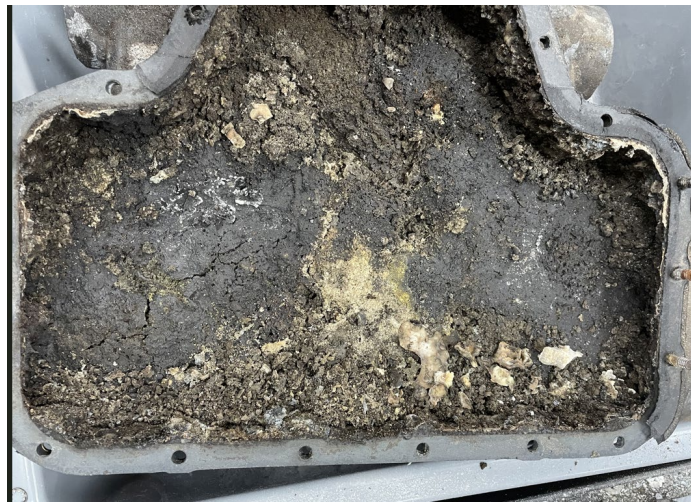
Figure 1: Lower oil sump with sludge
