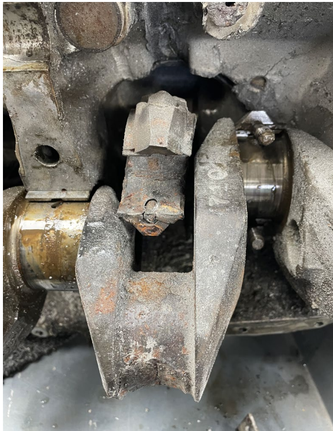
Figure 5: Cylinder 2 connecting rod end and cylinder 2 crankshaft journal
