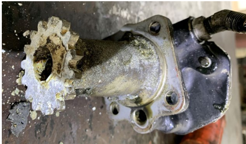
Figure 8: View of oil pump and impeller.
