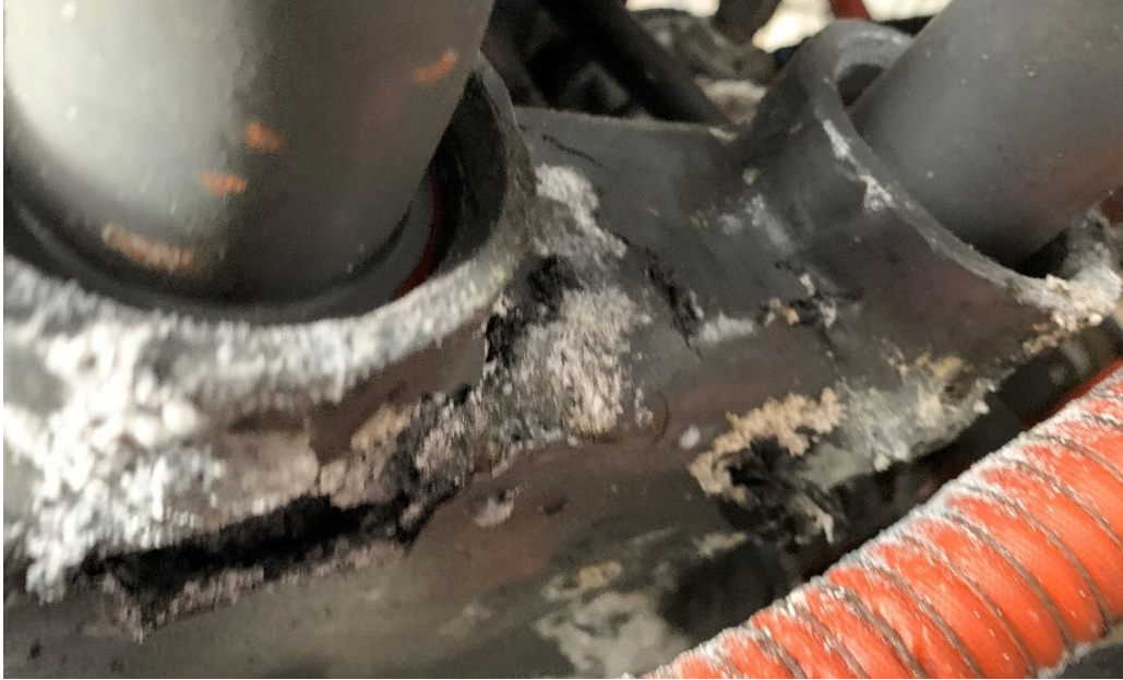
Figure 7: Hole in oil sump near the no. 2 cylinder induction tube.
