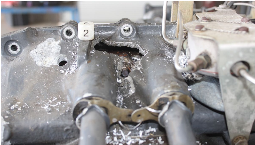
Figure 5: View of engine case breach.
