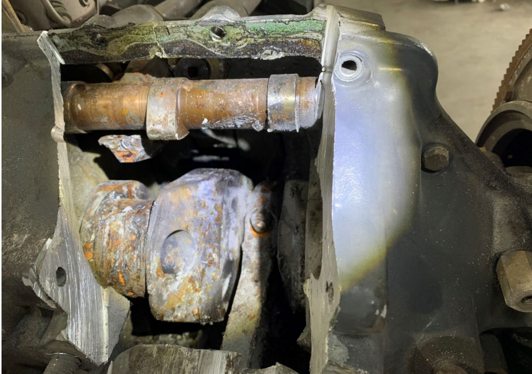
Figure 10: View of internal damage to the connecting rod and crankshaft journal.
